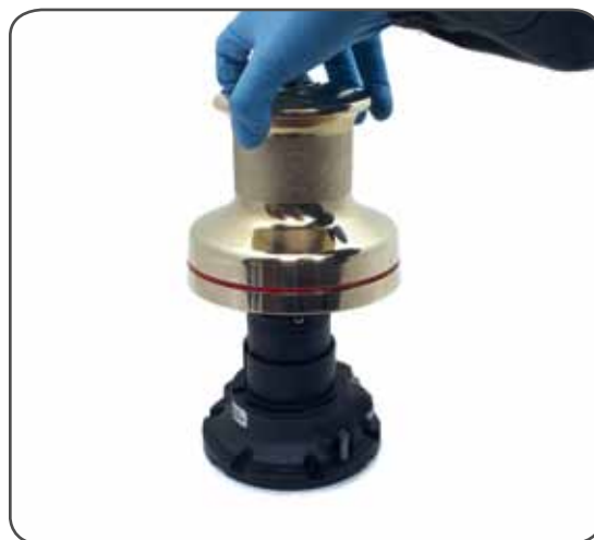
2. Lift off the drum n°12 with the socket n°18
