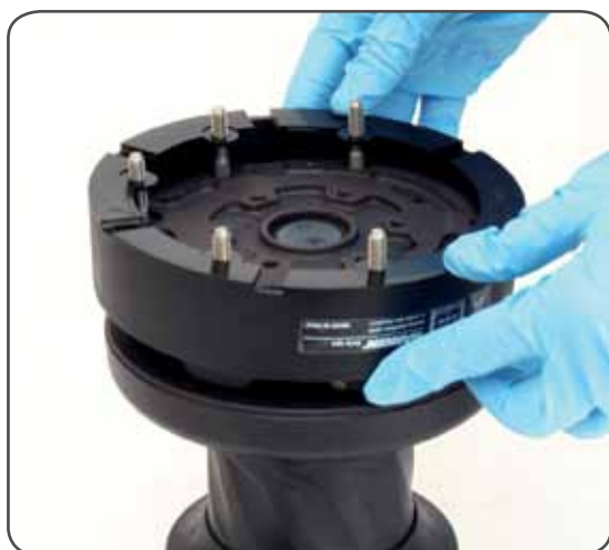
4. Reposition the skirt n°2 in its housing
