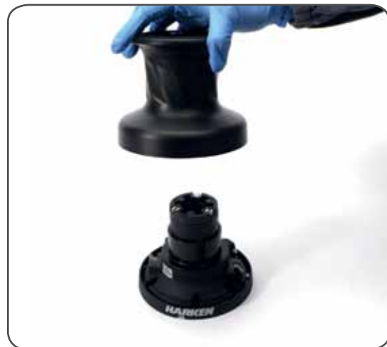
2. Lift off the drum n°13 with the socket n°17 and the washer n°20. Important: pay attention to the pawls n°4 inside the plain top.
