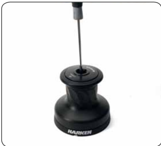
1. Unscrew the central screw ( \approx 2\text{Nm}/18\text{ in-lb} )
