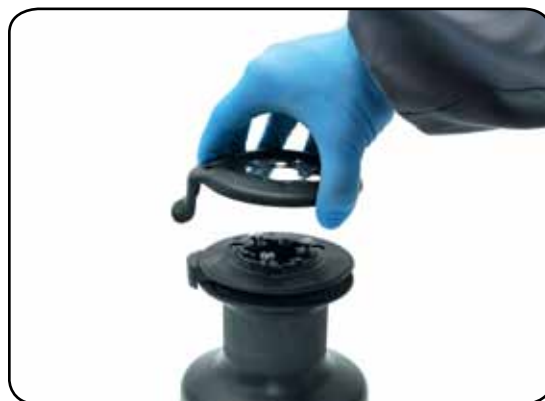
4. Remove the stripper arm n°15 by rotating and lifting it.
