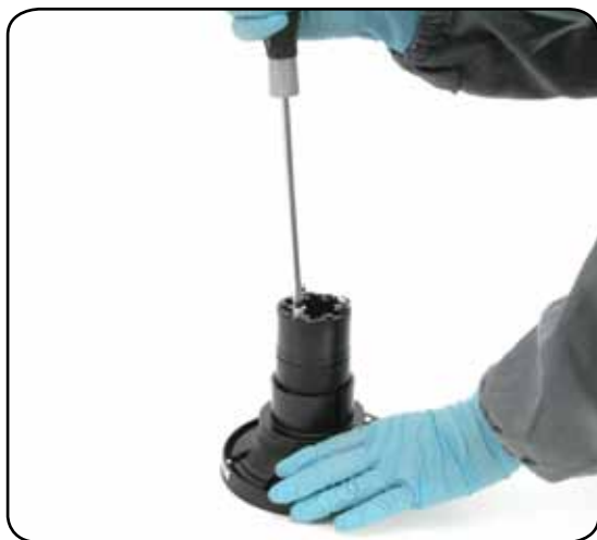
6. Completely unscrew the three screws n°16
