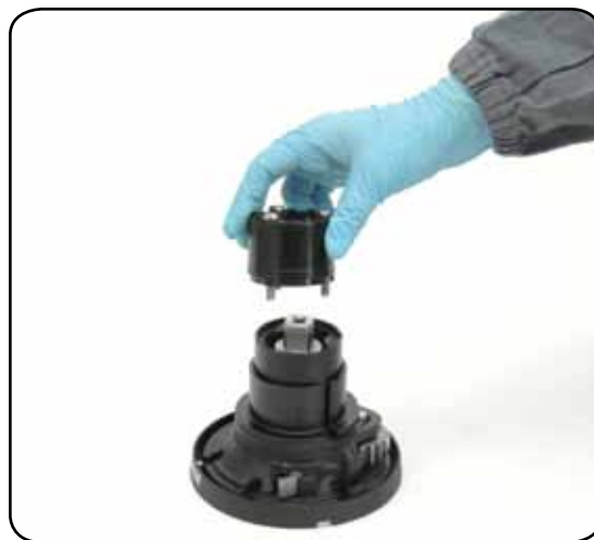
7. Remove the stripper arm support n°12 and slide out the bushing
