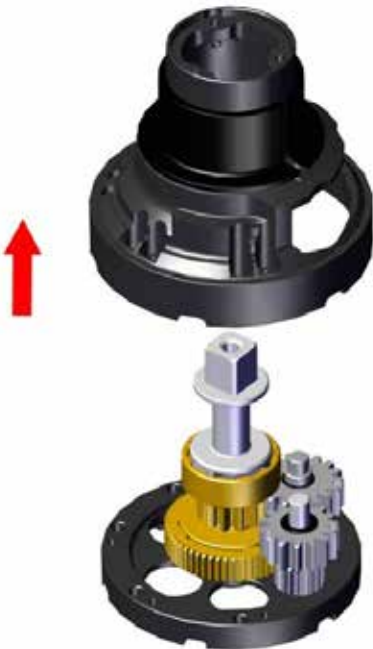
8. Slide out the drum support
