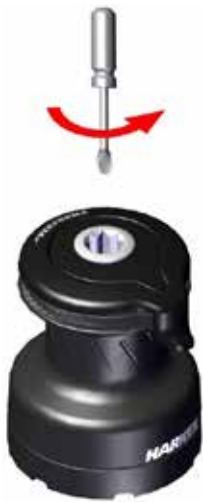
1. Unscrew the central screw ( \approx 2\text{Nm}/18\text{ in-lb} )
