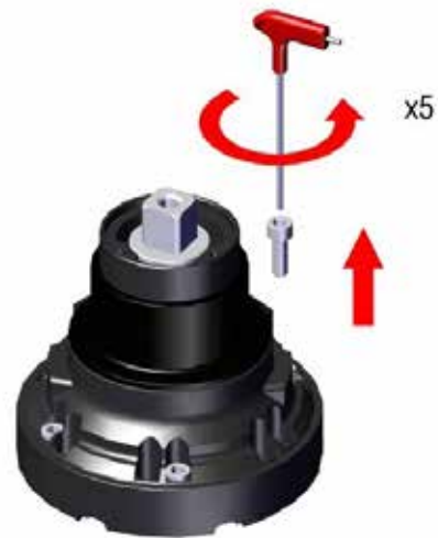
7. Unscrew the five drum support screws ( 20\text{Nm}/180\text{ in-lb} )
