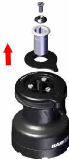
2. Slide off the socket and the cover
