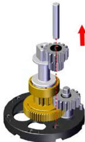
9. Slide out the pin and the gear
