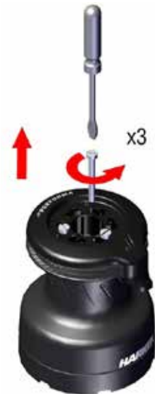
3. Unscrew the three screws ( \approx 4\text{Nm}/35\text{ in-lb} )
