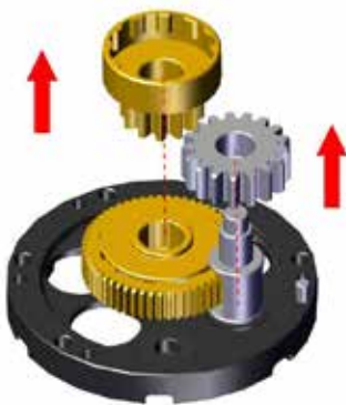
11. Slide out the central pawl carrier and the gear
