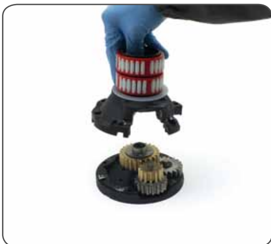
8. Remove the housing n°14 Important: washer n°11 may remain inside the housing!
