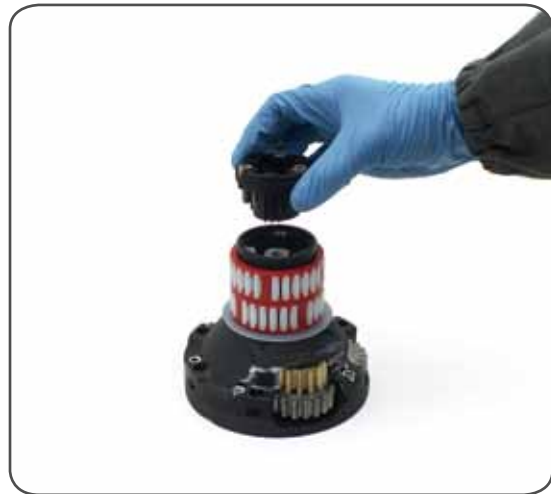
5. Remove the socket support n°20
