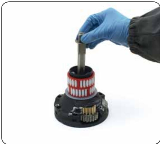
6. Slide out the central shaft n°18
