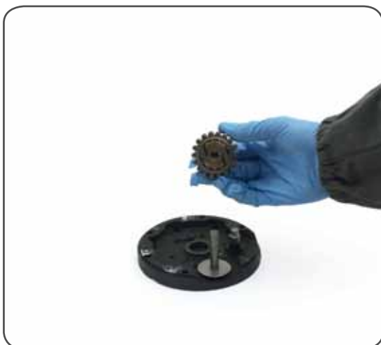
14. Remove the pinion n°10 and the pawls n°3. To facilitate the operation press the spring against the pawl with a blade.
