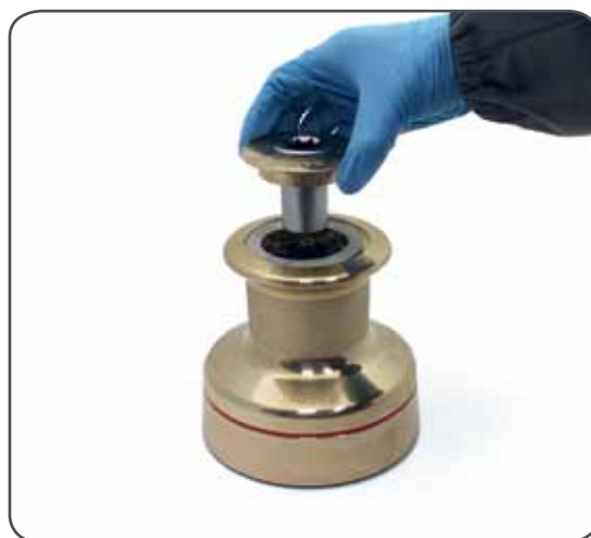
2. Slide off the socket n°29 and the cover n°25
