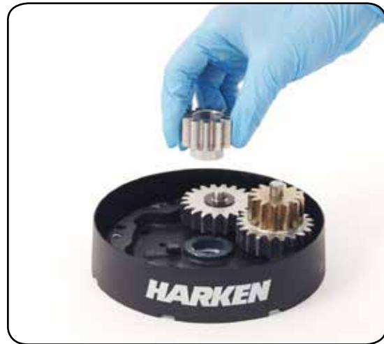
13. Remove the gear
