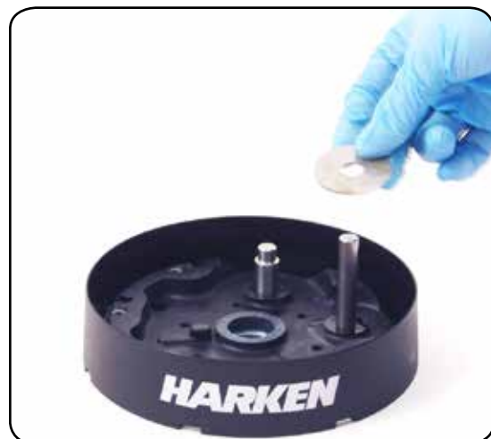
17. Remove the washer
