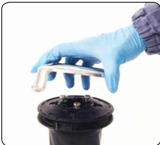
5. Remove the self-tailing arm by rotating and lifting it.
