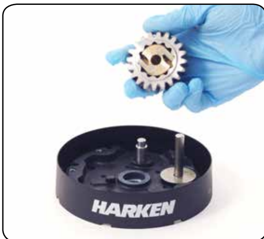
16. Remove the pawls carrier
