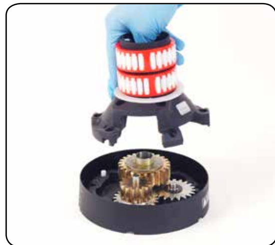
9. Remove the assy housing
