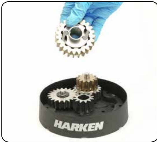
12. Remove the pawls carrier
