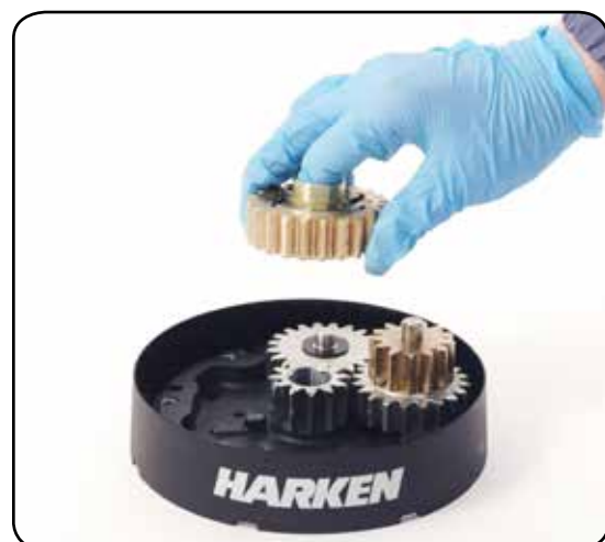
11. Remove the gear
