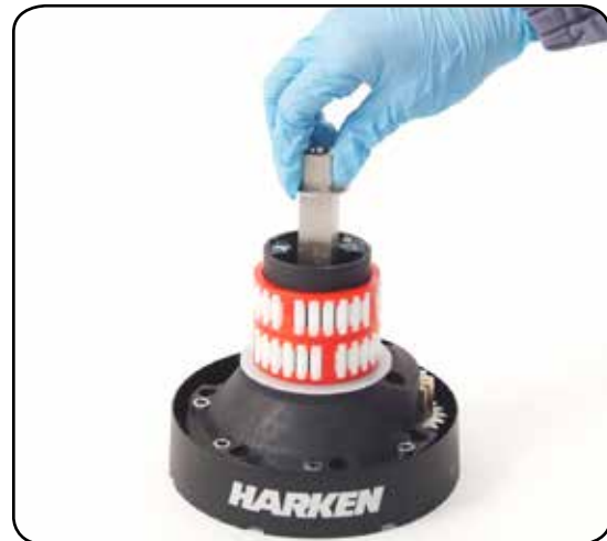
7. Slide out the central shaft
