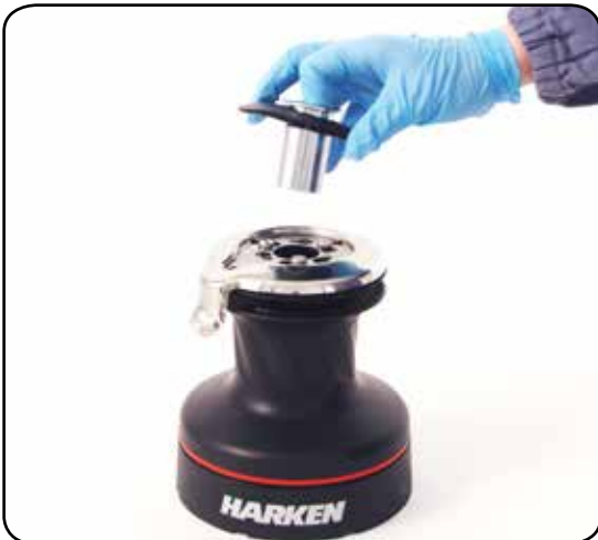
3. Slide off the assy socket and the cover. Pay attention to the o-ring in the socket.
