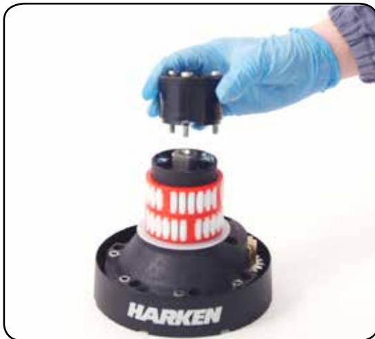
6. Completely unscrew the three screws and remove the stripper arm support
