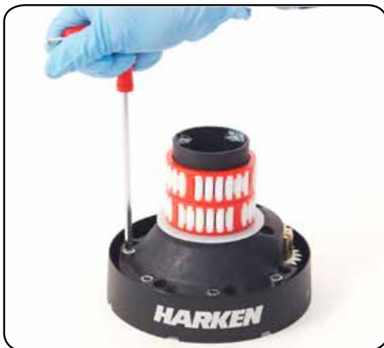
8. Unscrew the 6 hex screws (20Nm/177 in-lb)
