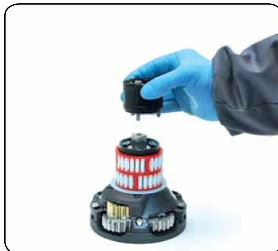
7. Remove the stripper arm support n°21
