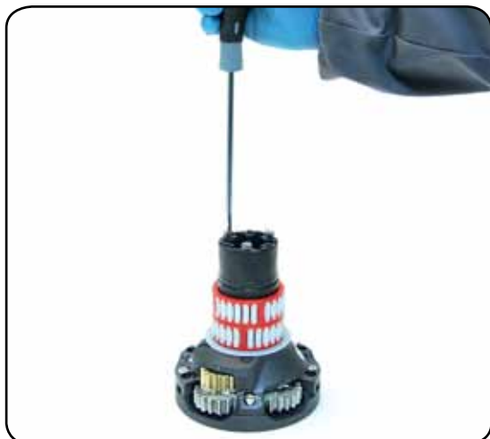
6. Completely unscrew the three screws n° 25
