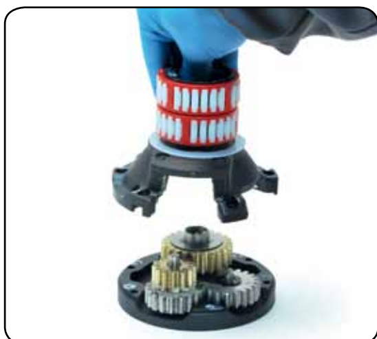
10. Remove the drum housing n°15 Important: washer n°12 may remain inside the drum housing!
