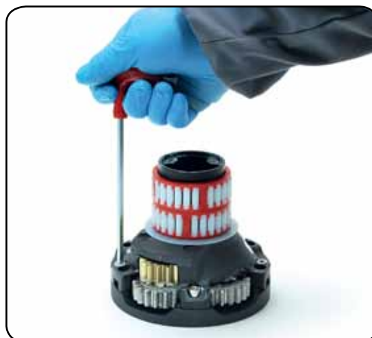
9. Unscrew the 6 hex screws n°16 (8Nm/71 in-lb)
