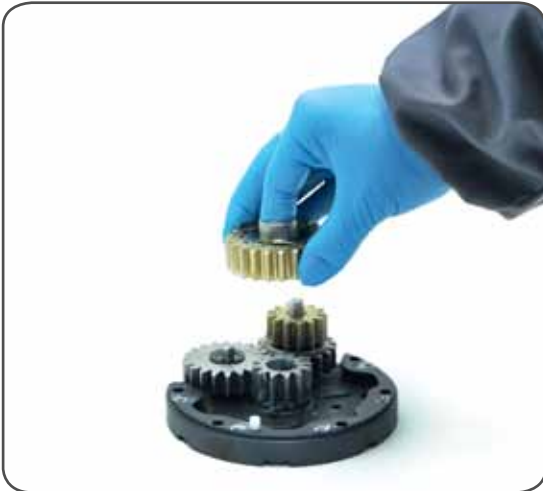
12. Remove gear n°7 and remove the pawls n°5. To facilitate the operation press the spring against the pawl with a blade.
