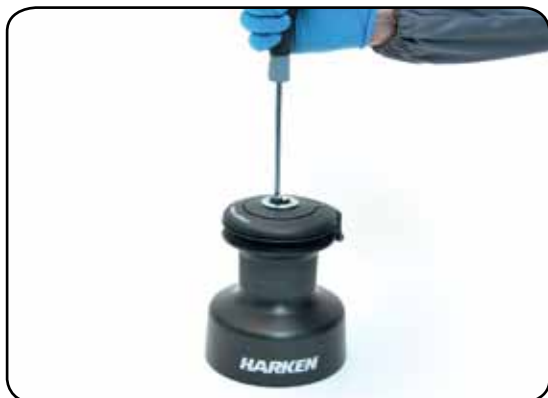
1. Unscrew the central screw ( \approx 2\text{Nm}/18\text{ in-lb} )
