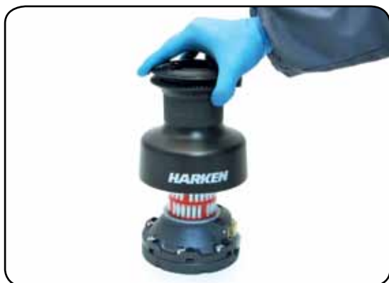
5. Lift off the drum n°29
