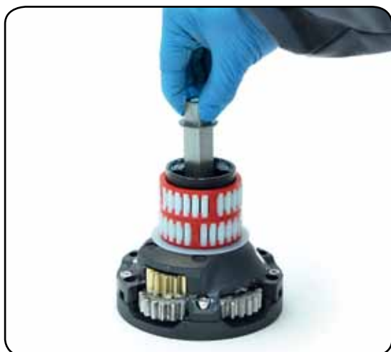
8. Slide out the central shaft n°19
