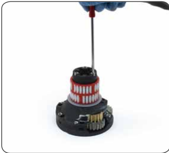
4. Completely unscrew the three screws n° 26
