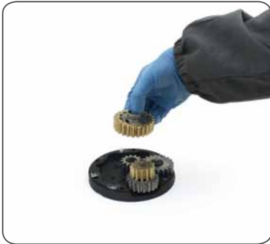
10. Remove the gear n°6 and remove the pawls n°3. To facilitate the operation press the spring against the pawl with a blade.
