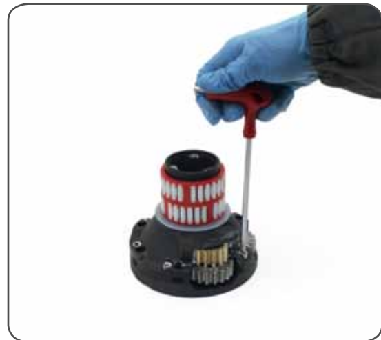
7. Unscrew the 6 hex screws n°15 ( \approx 8\text{Nm}/71\text{ in-lb} )
