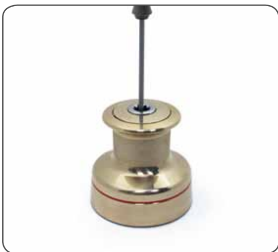
1. Unscrew the central screw ( \approx 2\text{Nm}/18\text{ in-lb} )
