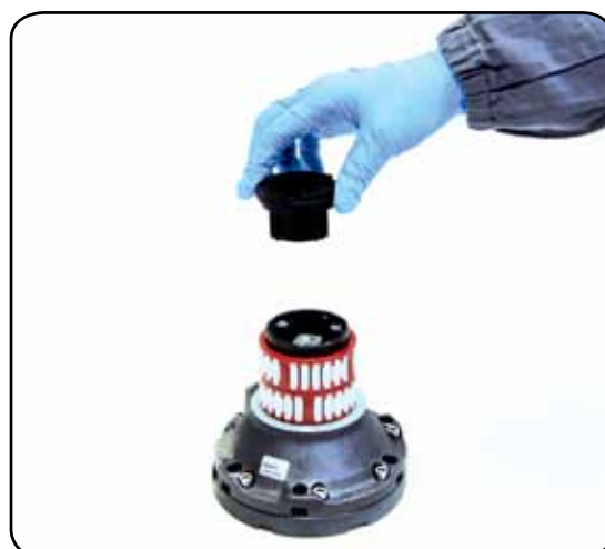
5. Remove the socket support n°20
