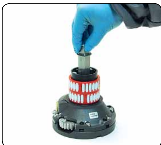
6. Slide out the central shaft n°18
