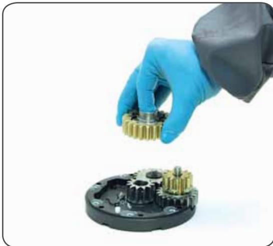
10. Remove the gearing n°6 and remove the pawls n°4. To facilitate the operation press the spring against the pawl with a blade.
