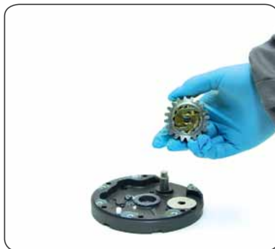
15. Remove the pawls n°4. To facilitate the operation press the spring against the pawl with a blade.
