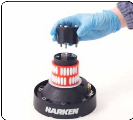
6. Completely unscrew the three screws; remove the stripper arm support
