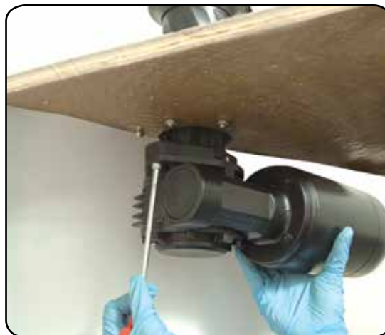
4. Tighten the two screws ( \approx 8 \text{ Nm} / 71 \text{ in-lb} ). Be sure to align the flange.
