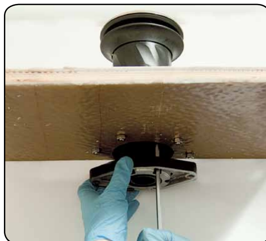
2. Tighten the six screws (8 Nm/ 71 in-lb)
