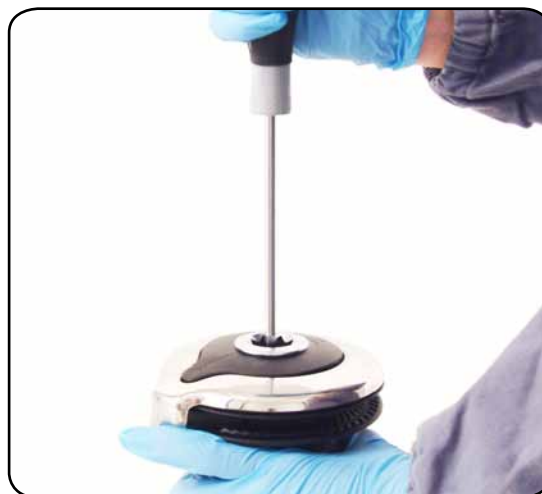
2. Unscrew the central screw ( \approx 2\text{Nm}/18\text{ in-lb} )
