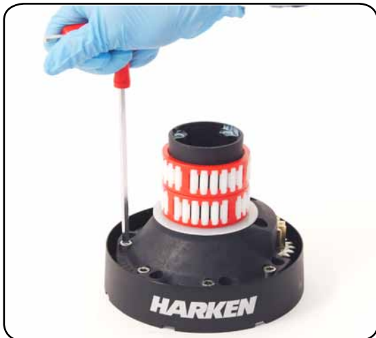
8. Unscrew the 5 hex screws n°16 ( \approx 20\text{Nm}/177\text{ in-lb} )
