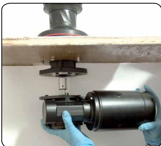
3. Position the reduction gear and motor
