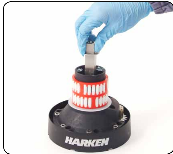
7. Slide out the central shaft n°19
