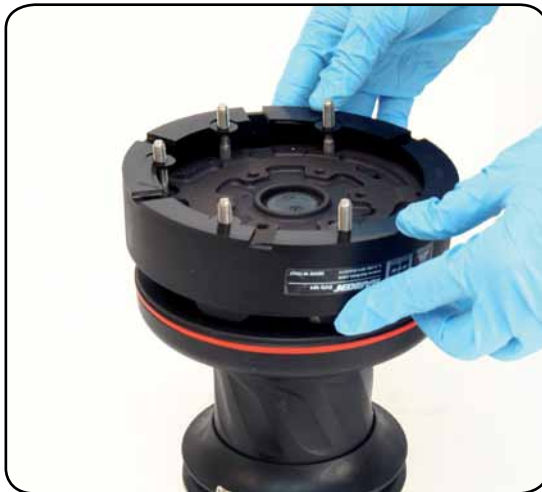
4. Reposition the skirt n°2 in its housing
