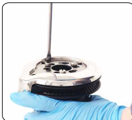
4. Unscrew the three screws n°27 ( \approx 4\text{Nm}/35\text{ in-lb} )
