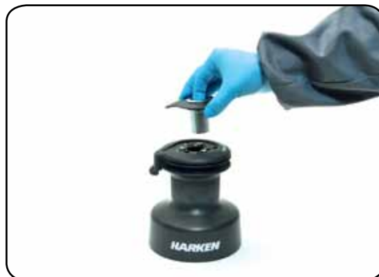
2. Slide off the socket n°25 and the cover n°26
