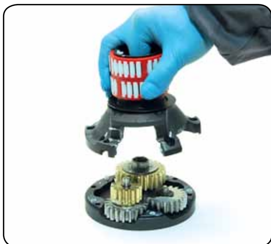
10. Remove the drum housing n°14 Important: washer n°11 may remain inside the drum support!
