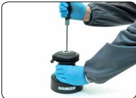
1. Unscrew the central screw ( \approx 2\text{Nm}/18\text{ in-lb} )
