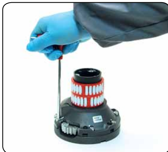
9. Unscrew the 6 hex screws n°15 ( \approx 8Nm/71 in-lb)
