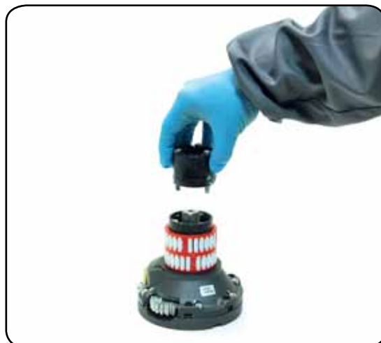
7. Remove the stripper arm support n°20
