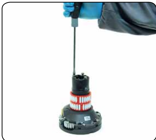
6. Completely unscrew the three screws n° 24
