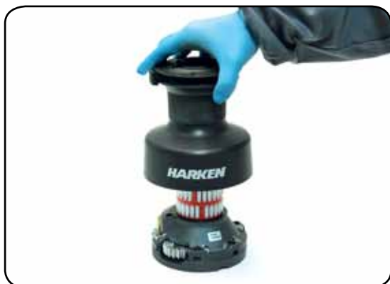
5. Lift off the drum n°21
