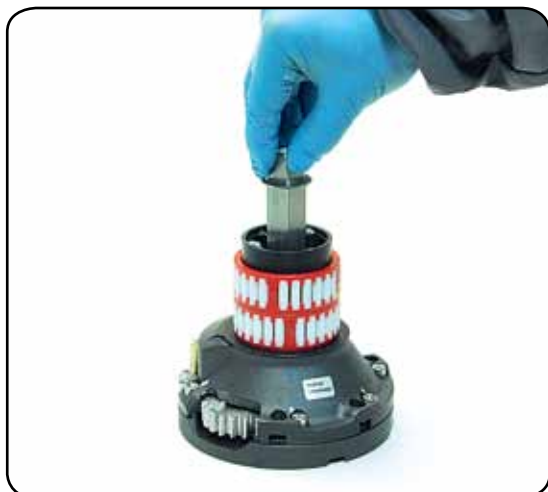
8. Slide out the central shaft n°18
