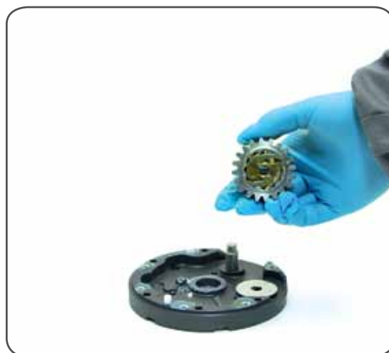
17. Remove the pawls n°4. To facilitate the operation press the spring against the pawl with a blade.
