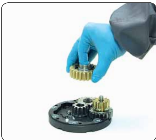
12. Remove gear n°6 and remove the pawls n°4. To facilitate the operation press the spring against the pawl with a blade.
