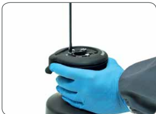
3. Unscrew the three screws n°24 ( \approx 4\text{Nm}/35\text{ in-lb} )
