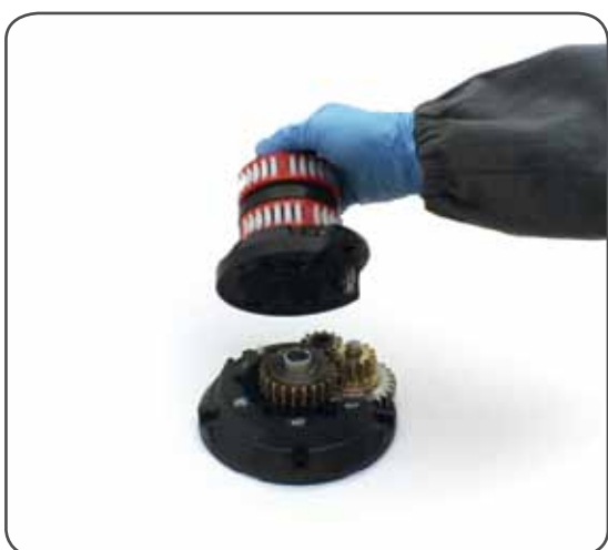
8. Remove the housing n°15 Important: washer n°12 may remain inside the housing!
