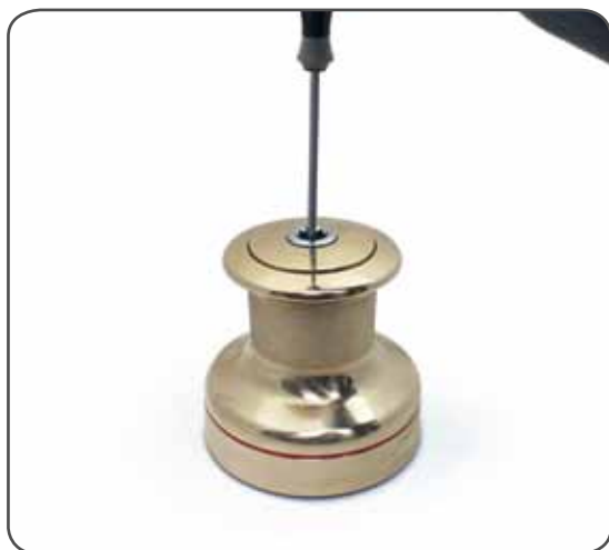
1. Unscrew the central screw ( \curvearrowright 2Nm/18 in-lb)
