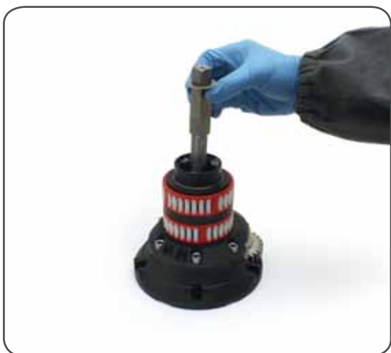
6. Slide out the central shaft n°19
