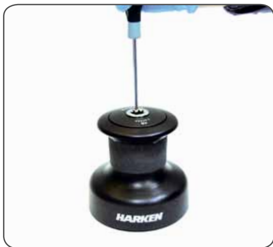
1. Unscrew the central screw (⚙️ 2Nm/18 in-lb)
