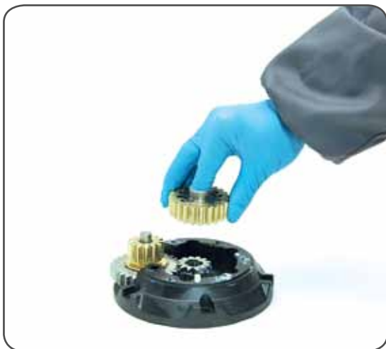
10. Remove the gearing n°9 and remove the pawls n°7. To facilitate the operation press the spring against the pawl with a blade.
