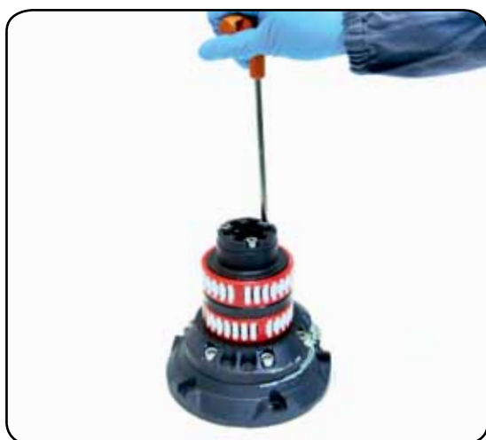
4. Completely unscrew the three screws n° 25 and remove the socket support
