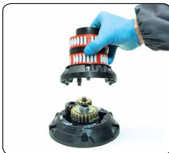
7. Remove the assy housing n° 15. Important: washer n° 12 may remain inside the drum support and the washer n° 29 must be replaced in the correct position.
