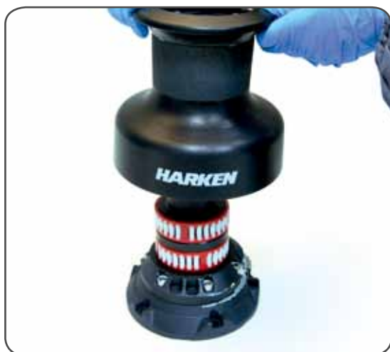
3. Lift off the drum n°22
