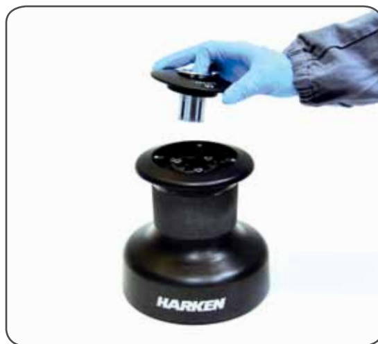
2. Slide off the hub n°27 and the cover n°26 and the washer n°30
