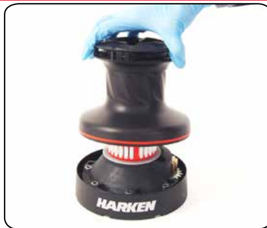
6. Lift off the drum
