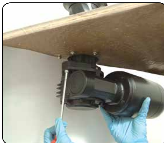
4. Tighten the two screws ( \approx 8 Nm/ 71in-lb). Be sure to align the flange.
