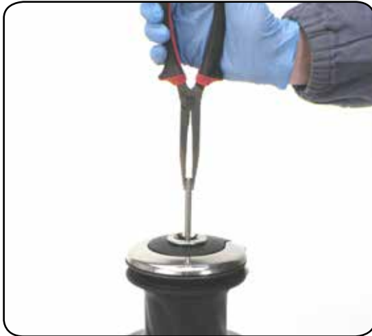
1. Pull out the disconnect rod
