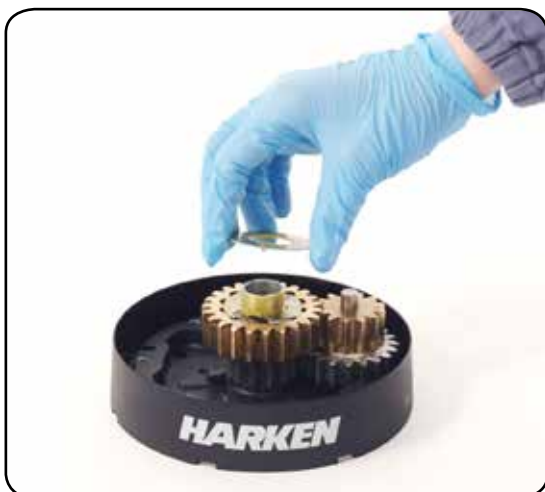
10. Remove the washer
