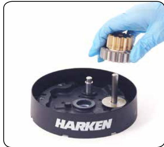
15. Remove the gear
