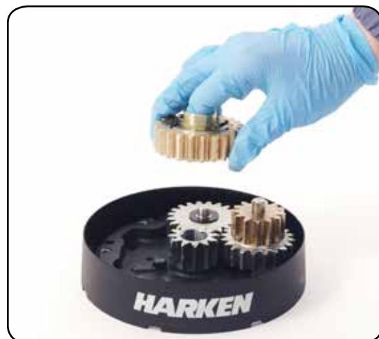
11. Remove the gear
