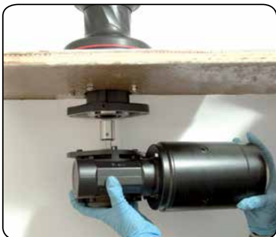
3. Position the reduction gear and motor
