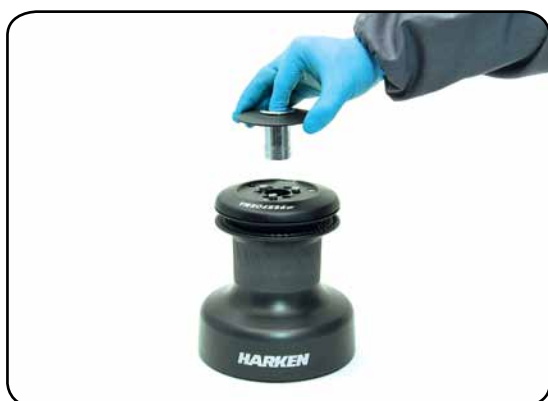
3. Slide off the assy socket n°27 and the cover n°26. Pay attention to the o-ring in the socket.
