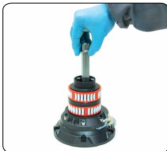
8. Slide out the central shaft n°19
