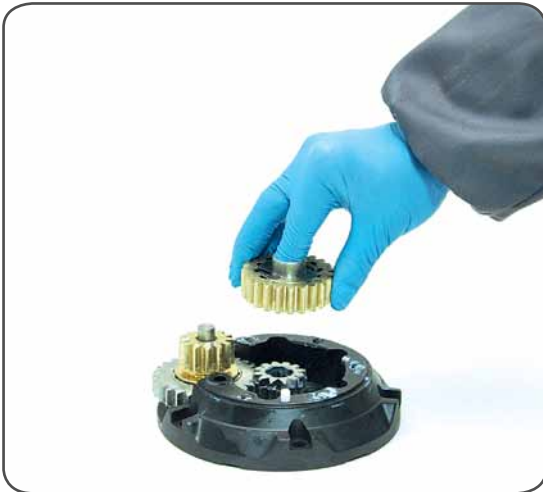
13. Remove the gearing n°9 and remove the pawls n°7. To facilitate the operation press the spring against the pawl with a blade.
