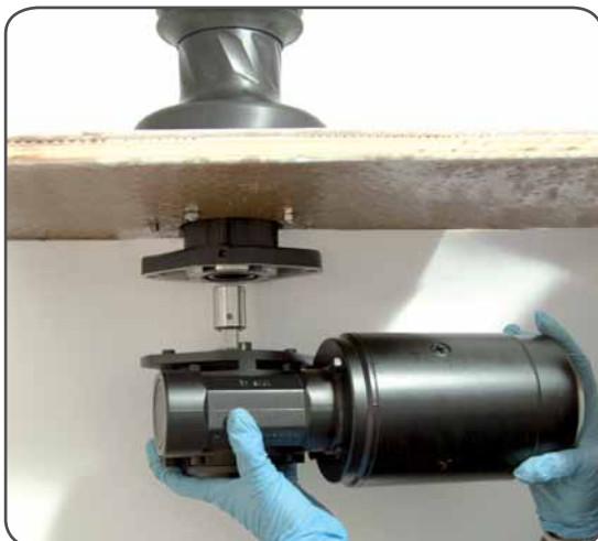
3. Position the reduction gear and motor
