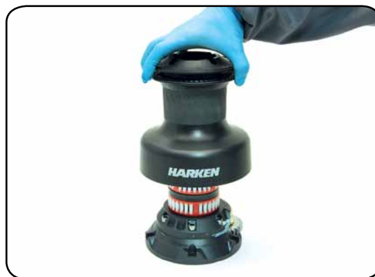
6. Lift off the drum n°28
