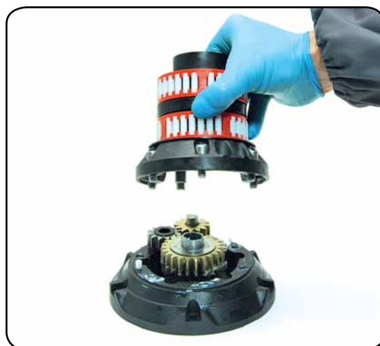
10. Remove the assy housing n°15 Important: washer n°12 may remain inside the drum support!
