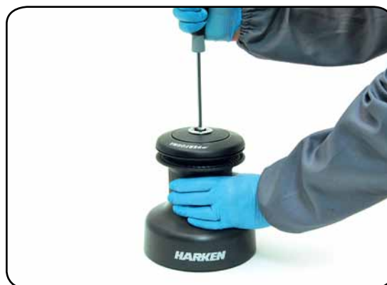
2. Unscrew the central screw ( \approx 2Nm/18 in-lb)
