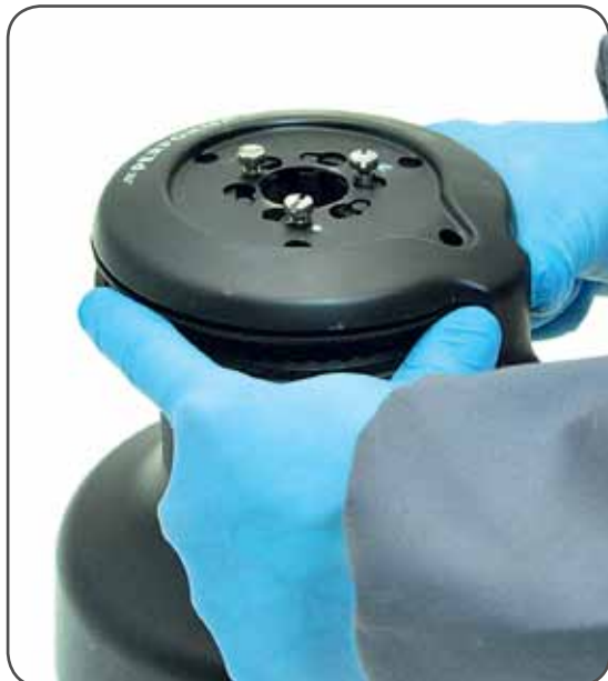
If the jaws have been disassembled, insert peeler between the two jaws, taking care that the letters TOP on the peeler are facing upwards.
