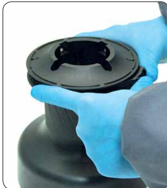
When positioning the stripper arm, align the peeler with it.
