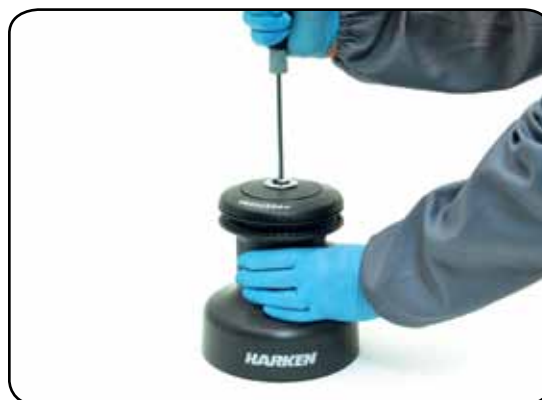
2. Unscrew the central screw ( \approx 2\text{Nm}/18\text{ in-lb} )
