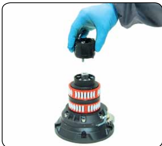
7. Completely unscrew the three screws n° 25 and remove the stripper arm support n°21
