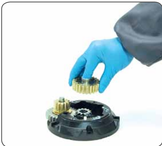
12. Remove gear n°9 and remove the pawls n°7. To facilitate the operation press the spring against the pawl with a blade.
