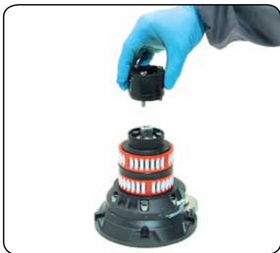
6. Completely unscrew the three screws n° 26 and remove the stripper arm support n°21
