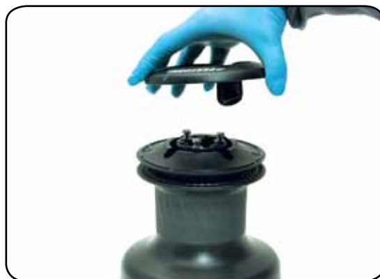
4. Remove the stripper arm n°24 by rotating and lifting it.
