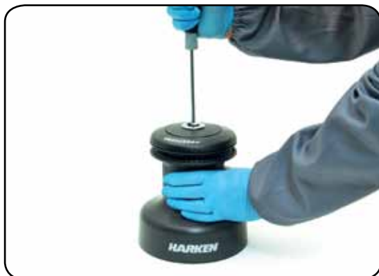
1. Unscrew the central screw ( \approx 2\text{Nm}/18\text{ in-lb} )
