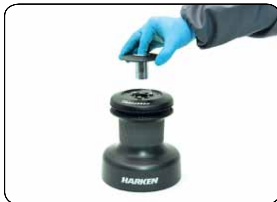
2. Slide off the assy socket n°27 and the cover n°26
