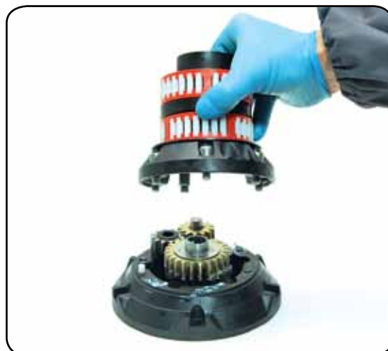
9. Remove the assy housing n°15 Important: washer n°13 may remain inside the drum support!
