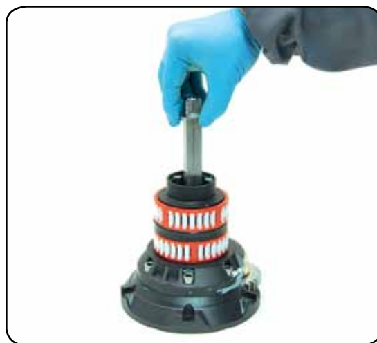
7. Slide out the central shaft n°19
