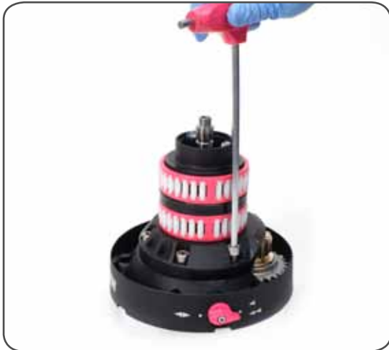
7. Unscrew the 5 hex screws n°12 ( \approx 20\text{Nm}/177\text{ in-lb} )
