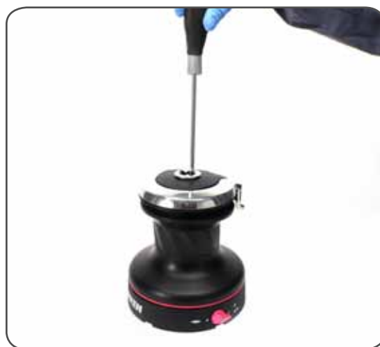
2. Unscrew the central screw ( \approx 2\text{Nm}/18\text{ in-lb} )
