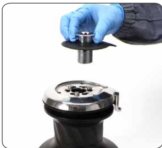
3. Slide off the assy socket n°37 and the cover n°38. Pay attention to the o-ring in the socket.
