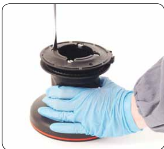
I. Unscrew the 4 screws n°18 ( \approx 4Nm/35 in-lb)
