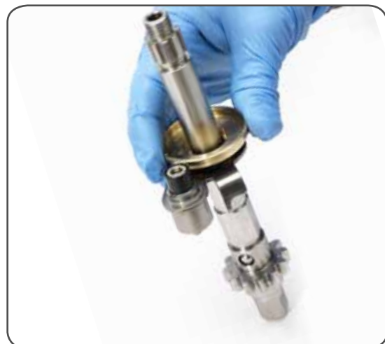
12. Slide out the command group and pay attention to the two balls n°23
