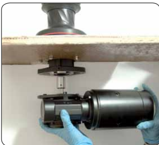
3. Position the reduction gear and motor
