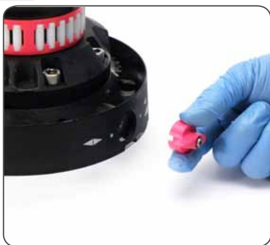
1. Unscrew the screw n°36 and slide off the knob (0,5 Nm/ 4,42 in-lb)
