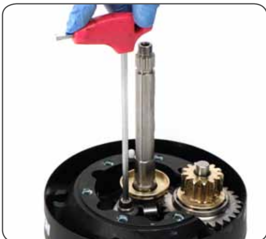
11. Unscrew the screw n°30 and slide out the main shaft n°21
