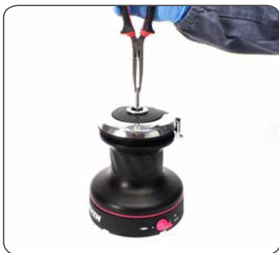
1. Pull out the disconnect rod n°28
