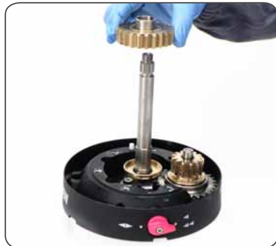
10. Remove gear n°27. Pay attention to the springs.
