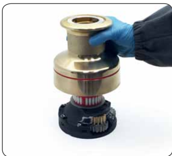
3. Lift off the drum n°23
