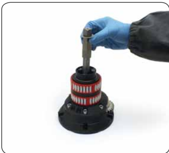
6. Slide out the central shaft n°20
