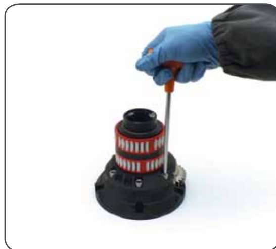
7. Unscrew the 5 hex screws n°17 ( \approx 8\text{Nm}/71\text{ in-lb} )
