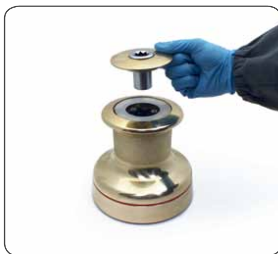
2. Slide off the assy socket n°31 and the cover n°29
