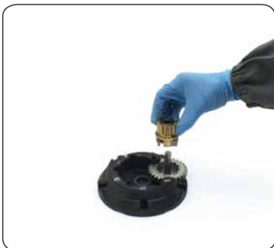
13. Remove the pinion n°10. To facilitate the operation press the spring against the pawl with a blade.
