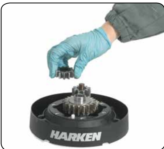
10. Remove the gear
