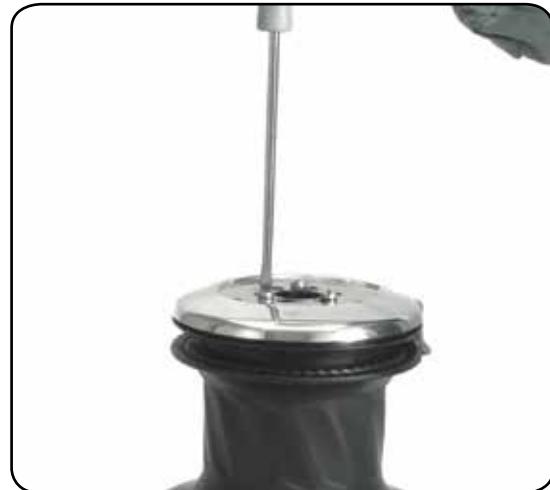
4. Unscrew the three screws ( \approx 4\text{Nm}/35\text{ in-lb} )
