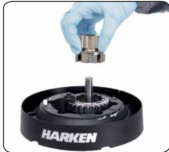
15. Remove the pinion.
