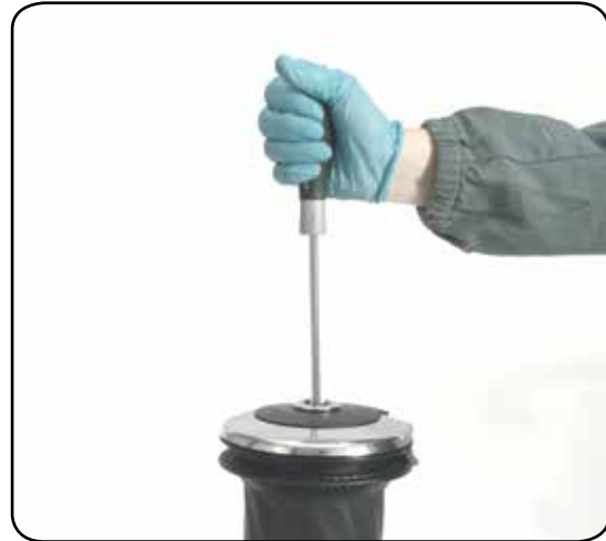
2. Unscrew the central screw ( \approx 2\text{Nm}/18\text{ in-lb} )
