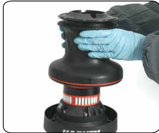
6. Lift off the drum
