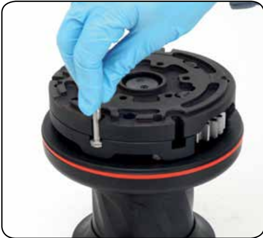
3. Position the five M8 hexagonal headed bolts in their holes
