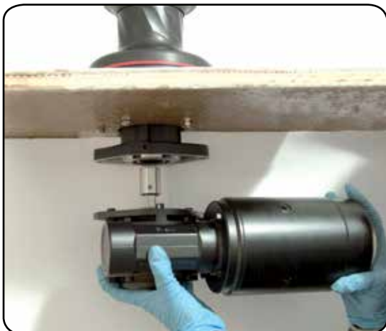
3. Position the reduction gear and motor
