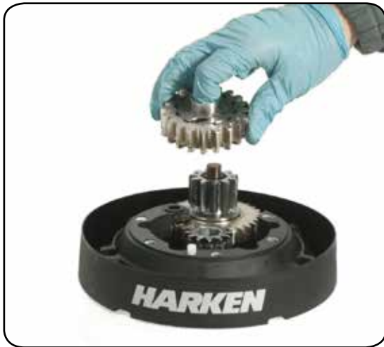
12. Remove the gear
