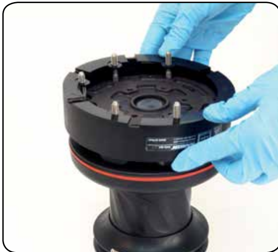
4. Reposition the skirt in its housing
