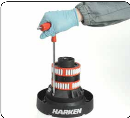
8. Unscrew the five hex screws ( \approx 20\text{Nm}/177\text{ in-lb} )
