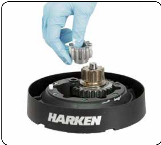
14. Remove the gear
