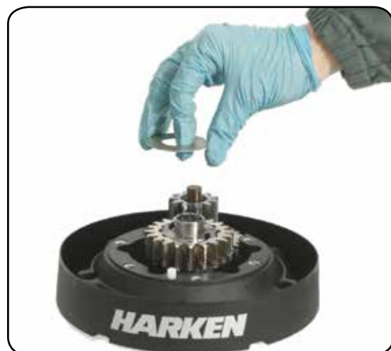
11. Remove the washer
