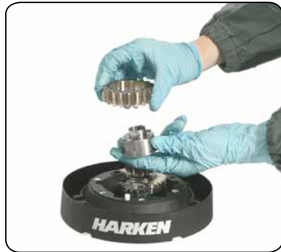
13. Remove the pawls carrier
