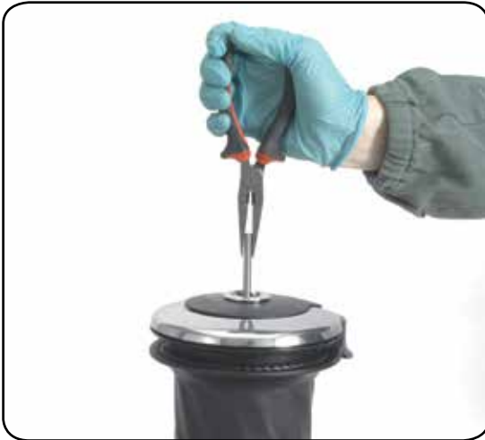
1. Pull out the disconnect rod
