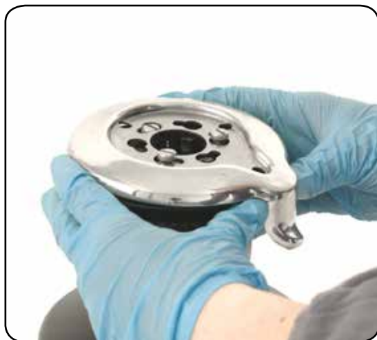
When positioning the stripper arm, align the peeler with it.
