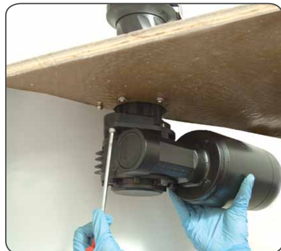
4. Tighten the two screws ( \approx 8 \text{ Nm} / 71 \text{ in-lb} ). Be sure to align the flange.
