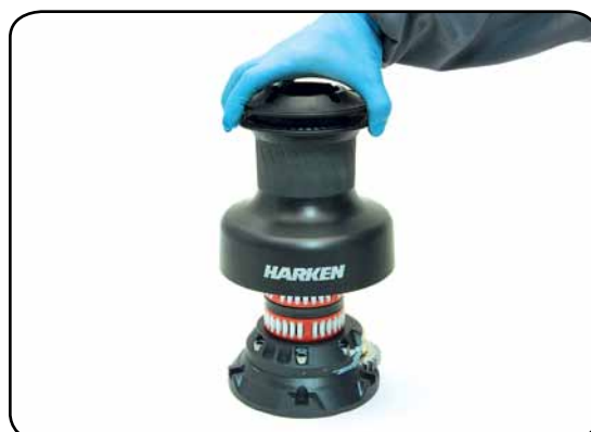
6. Lift off the drum n°23
