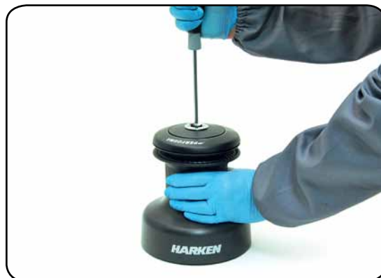
2. Unscrew the central screw ( \approx 2\text{Nm}/18\text{ in-lb} )
