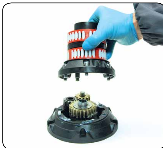
10. Remove the assy housing n°16 Important: washer n°13 may remain inside the drum support!
