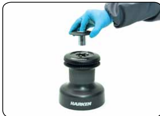
2. Slide off the assy socket n°29 and the cover n°28
