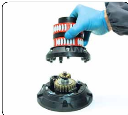
9. Remove the assy housing n°16 Important: washer n°13 may remain inside the drum support!
