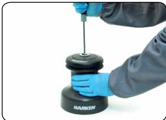
1. Unscrew the central screw ( \approx 2\text{Nm}/18\text{ in-lb} )
