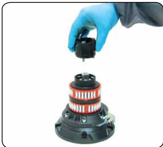
6. Completely unscrew the three screws n° 27 and remove the stripper arm support n°22
