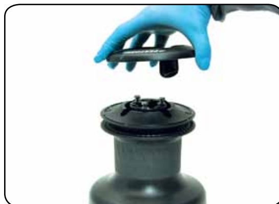
4. Remove the stripper arm n°26 by rotating and lifting it.
