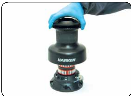
5. Lift off the drum n°23
