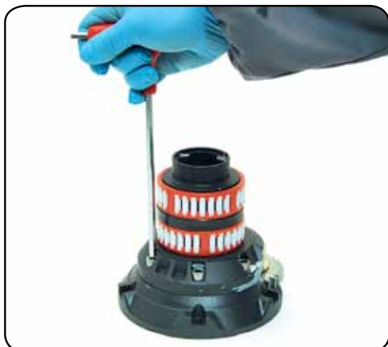
9. Unscrew the 5 hex screws n°17 ( \approx 20\text{Nm}/177\text{ in-lb} )
