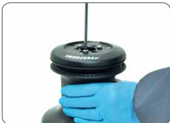
3. Unscrew the three screws n°27 ( \approx 4\text{Nm}/35\text{ in-lb} )
