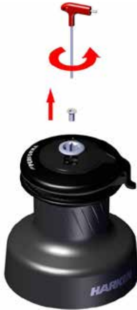
1. Unscrew the M8 central screw 40Nm
