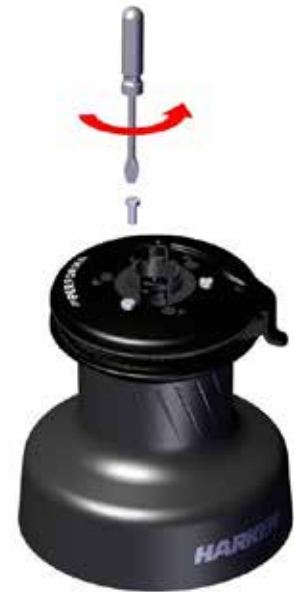
3. Unscrew the three M6 screws 16Nm
