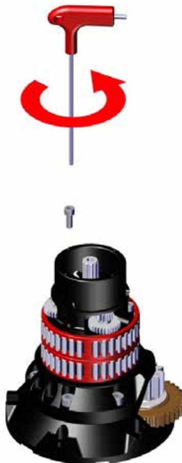
6. Unscrew the four M6 screws 16Nm
