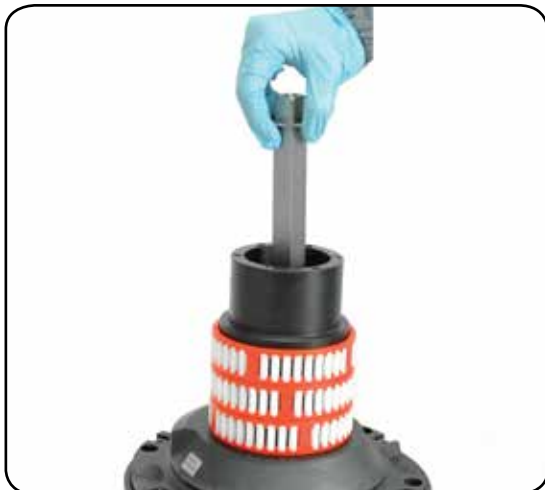
9. Slide out the central shaft
