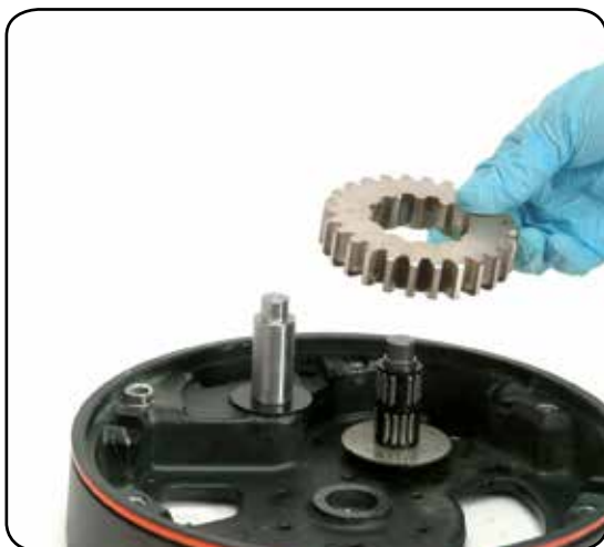
17. Remove the gear
