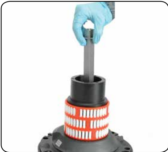
9. Slide out the central shaft
