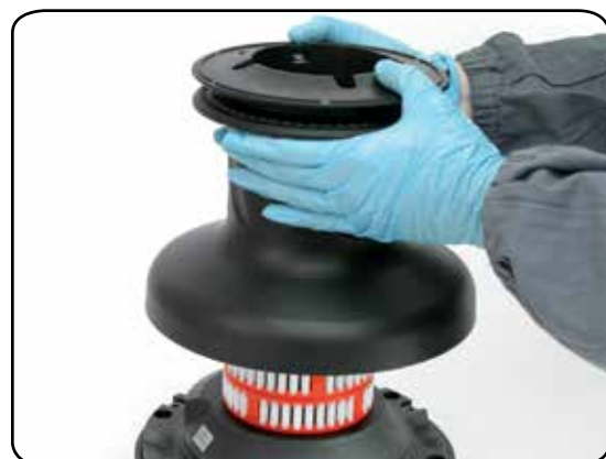
6. Lift off the drum
