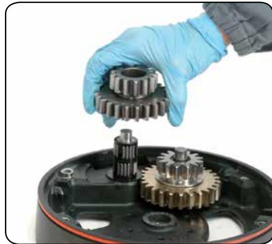
14. Remove the idler and pin
