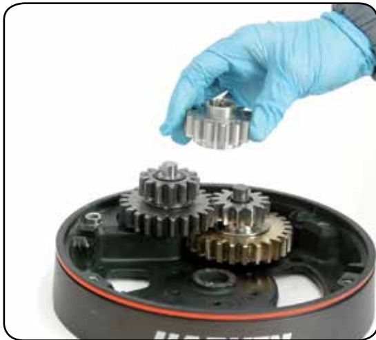
13. Remove the gear
