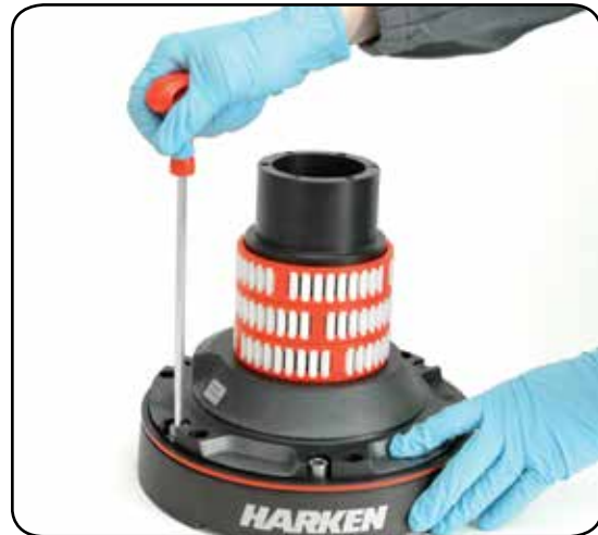
10. Unscrew the 6 hex screws ( 20Nm/177 in-lb)
