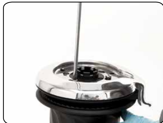
4. Unscrew the three screws ( \approx 4\text{Nm}/35\text{ in-lb} )
