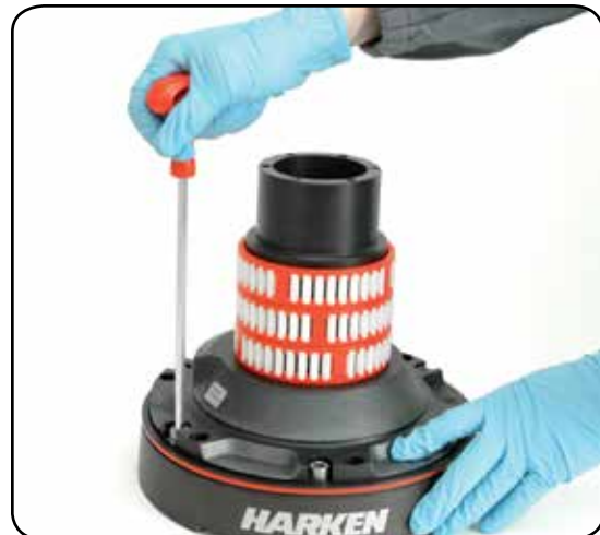
10. Unscrew the 6 hex screws ( 20Nm/177 in-lb)
