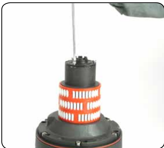
6. Completely unscrew the three screws n° 28
