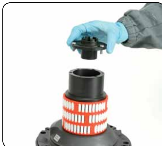
7. Remove the stripper arm housing n°21
