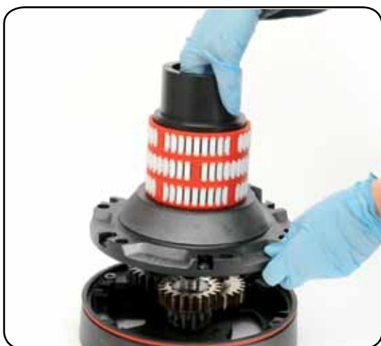
10. Remove the drum support n°16
