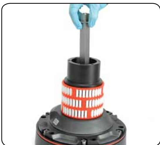
8. Slide out the central shaft n°19
