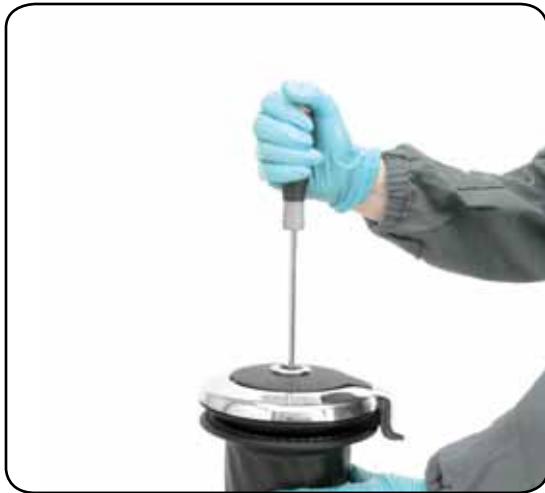
1. Unscrew the central screw (⚙️ 2Nm/18 in-lb)
