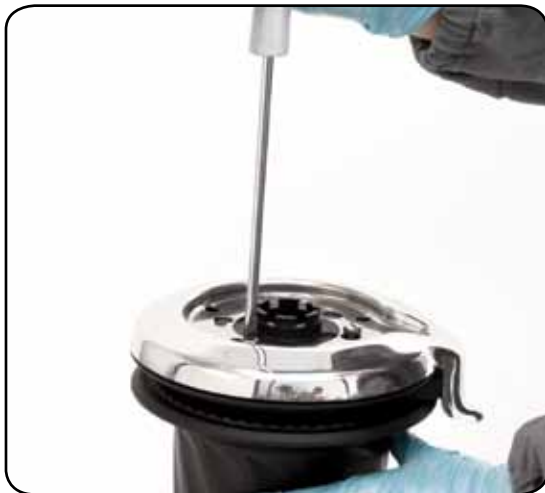
3. Unscrew the three screws n°28 (⚙️ 4Nm/35 in-lb)
