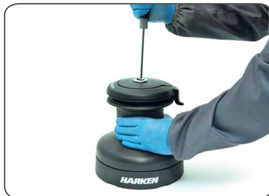
2. Unscrew the central screw ( \approx 2\text{Nm}/18\text{ in-lb} )
