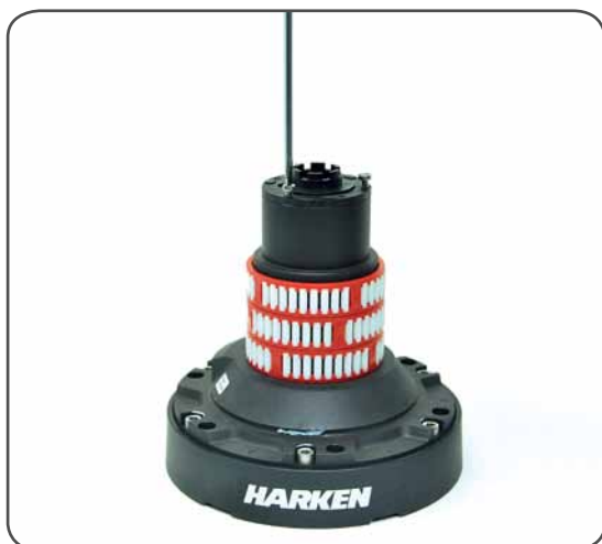
7. Completely unscrew the three screws n° 27
