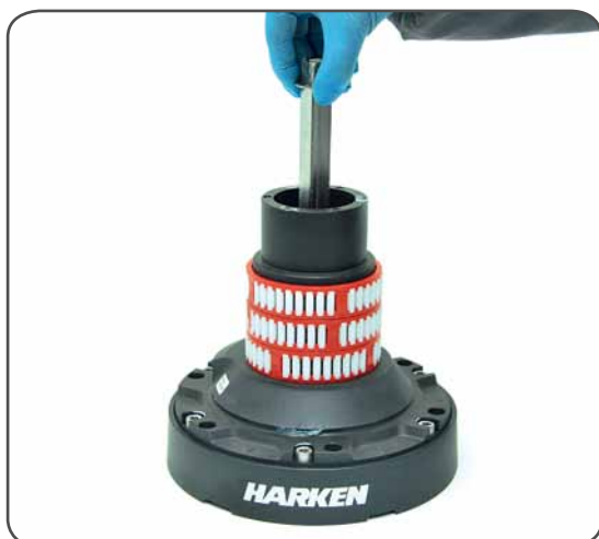
9. Slide out the central shaft n°19
