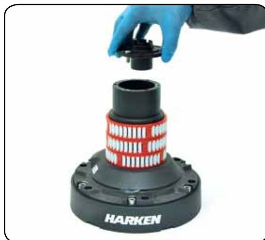
7. Remove the stripper arm housing n°21
