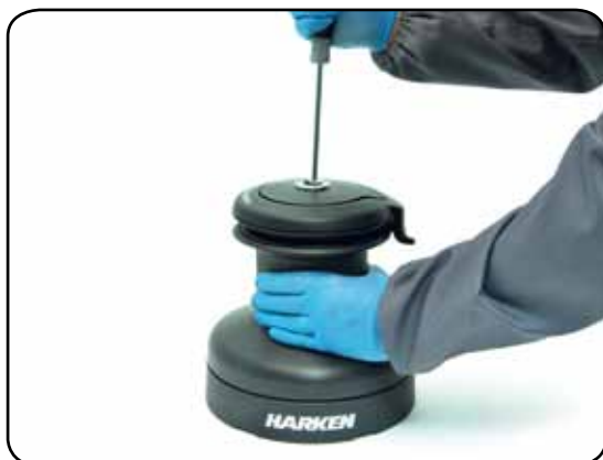
1. Unscrew the central screw ( \approx 2\text{Nm}/18\text{ in-lb} )
