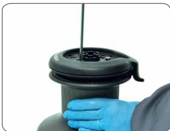
3. Unscrew the three screws n°26 ( \approx 4\text{Nm}/35\text{ in-lb} )
