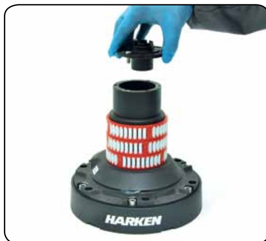
7. Remove the stripper arm housing n°21
