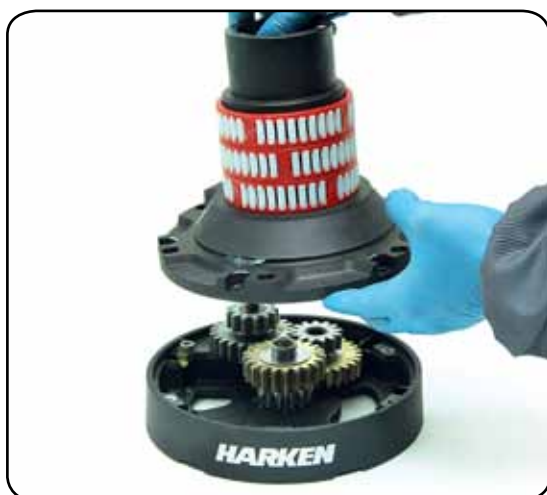
10. Remove the assy housing n°16
