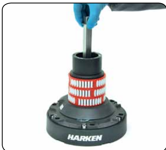
8. Slide out the central shaft n°19
