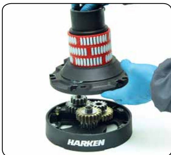
10. Remove the assy housing n°16
