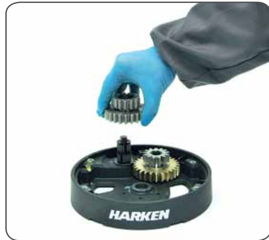
13. Remove the idler and pinion n°14.
