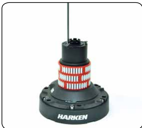
6. Completely unscrew the three screws n° 26
