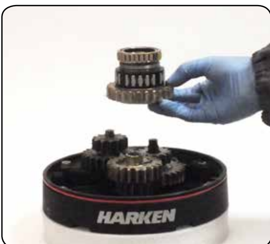
12. Remove the gear, pawls carrier, the bearings and the spring
