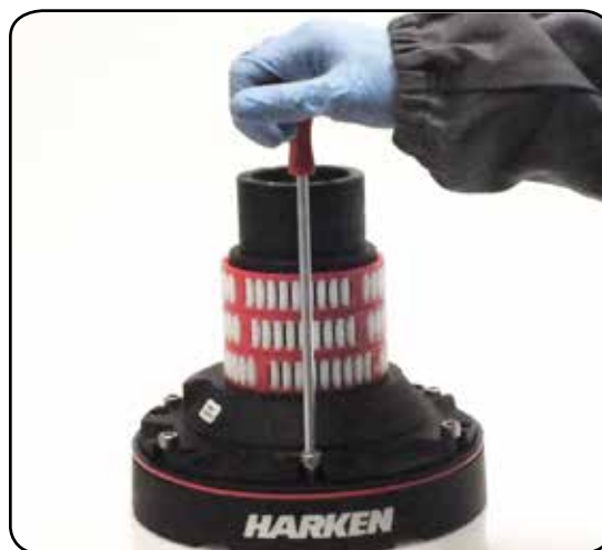
10. Unscrew the 6 hex screws ( \approx 20\text{Nm}/177\text{ in-lb} )
