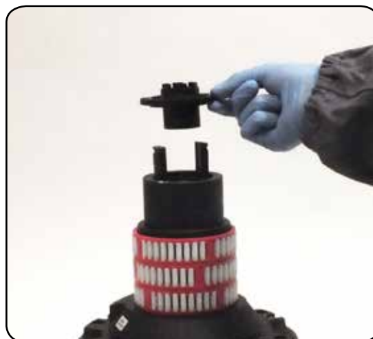
7. Remove the stripper arm housing
