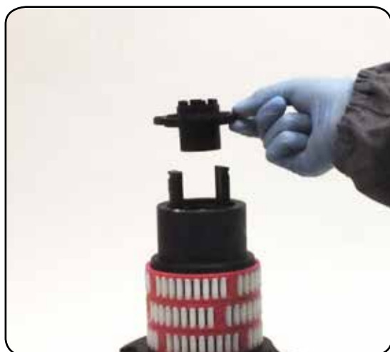
7. Remove the stripper arm housing
