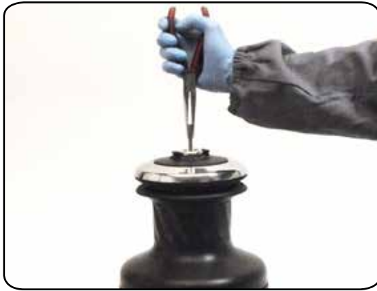
1. Pull out the disconnect rod
