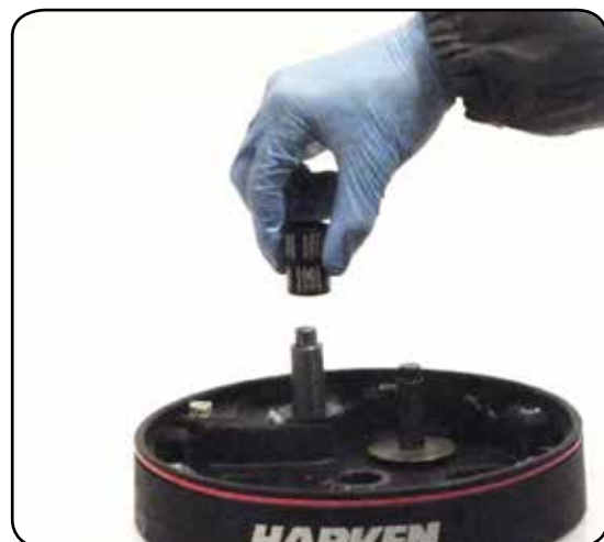
18. Remove roller bearings
