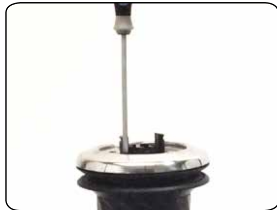
4. Unscrew the three screws ( \approx 4\text{Nm}/35\text{ in-lb} )
