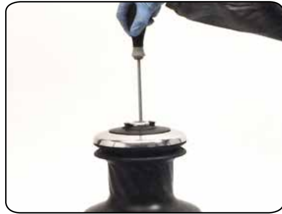
2. Unscrew the central screw ( \approx 2\text{Nm}/18\text{ in-lb} )
