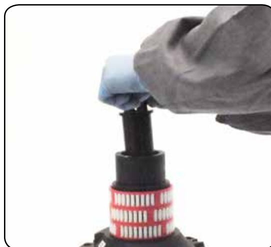
8. Slide out the assy clutch
