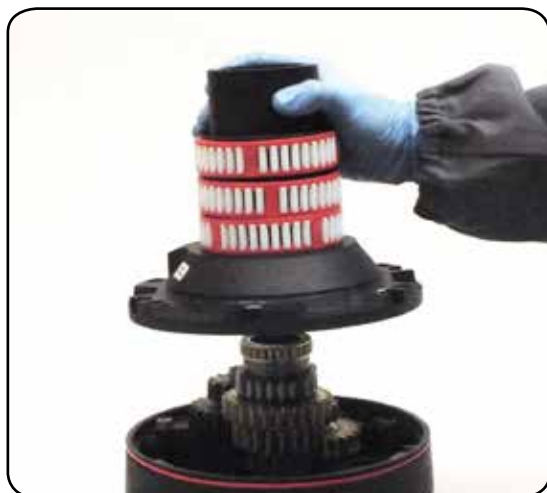
11. Remove the drum support
