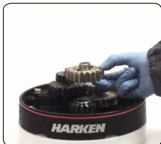
13. Remove the gear, pawls carrier and the washer
