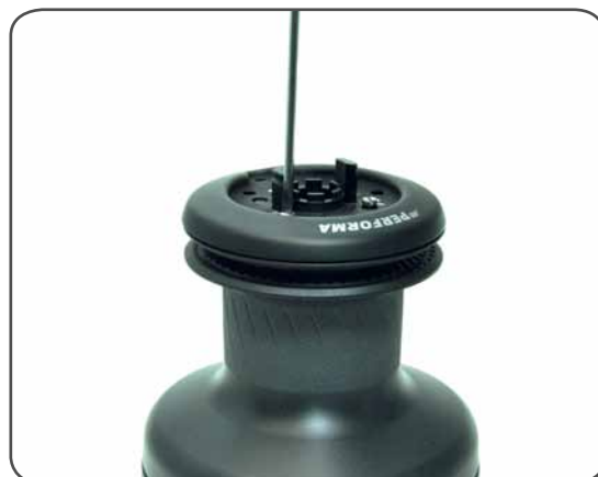
4. Unscrew the three screws n°27 ( \approx 4\text{Nm}/35\text{ in-lb} )
