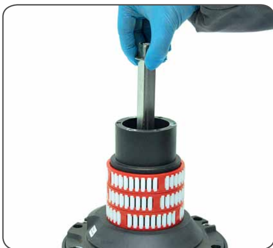
9. Slide out the central shaft n°19
