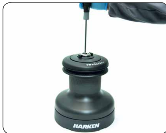
2. Unscrew the central screw ( \approx 2\text{Nm}/18\text{ in-lb} )
