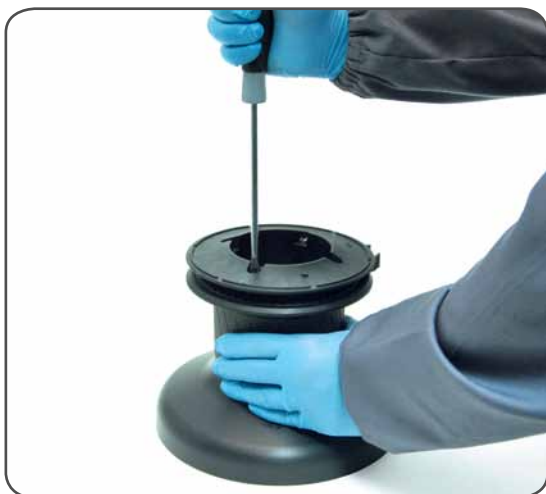
I. Unscrew the 4 screws n°25 (4Nm/35 in-lb)
