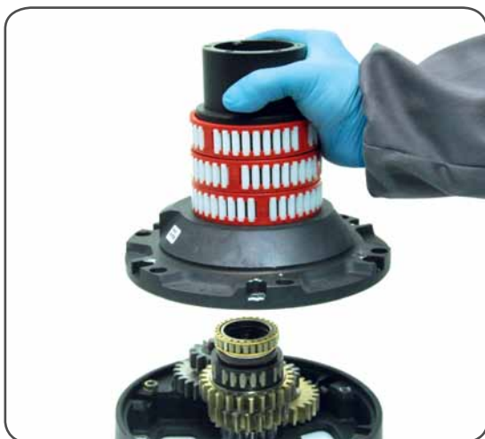
11. Remove the drum support n°16
