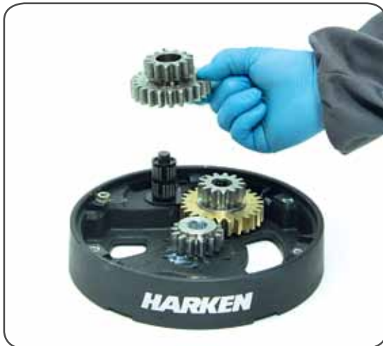
14. Remove the idler and pinion n°14
