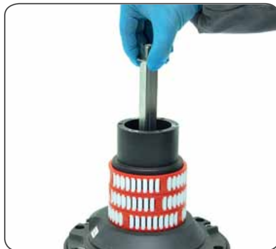
9. Slide out the central shaft n°19
