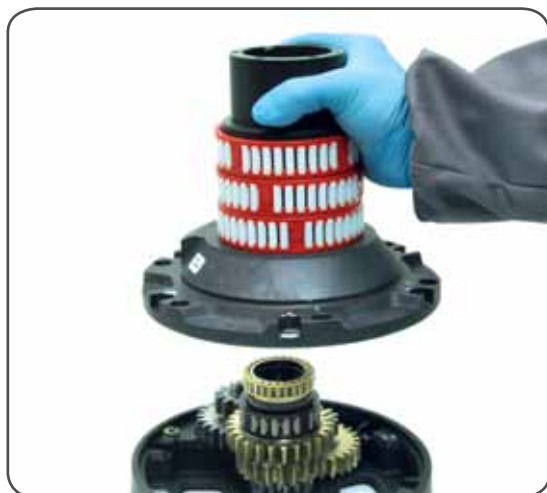
11. Remove the drum support n°16
