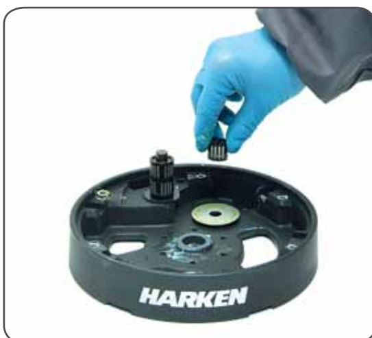
18. Remove the roller bearing n°12
