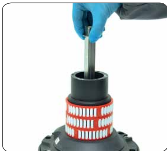
9. Slide out the central shaft n°19
