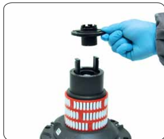
7. Remove the stripper arm housing n°21
