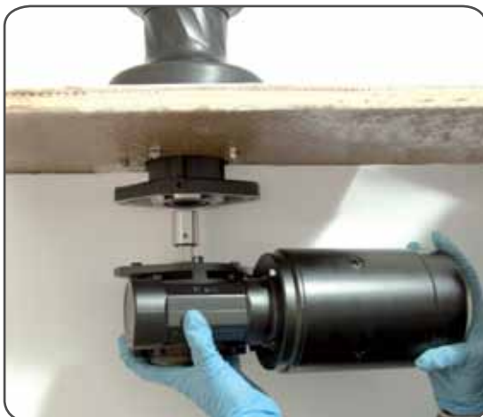
3. Position the reduction gear and motor
