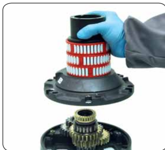
11. Slide out the drum support n°16
