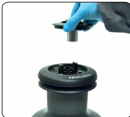
2. Slide off the assy socket n°28 and the cover n°27
