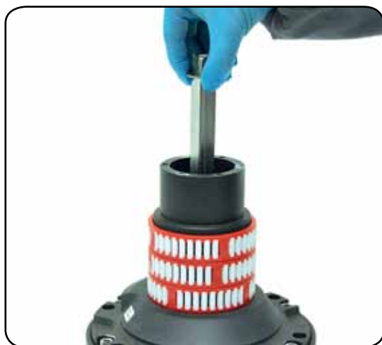
8. Slide out the central shaft n°19
