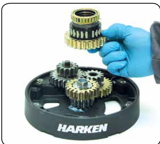
11. Remove the gear n°29, pawls carrier n°31, the bearings n°32 and 34 and the clutch spring n°33. Important: washer n°7 may remain inside the drum support!
