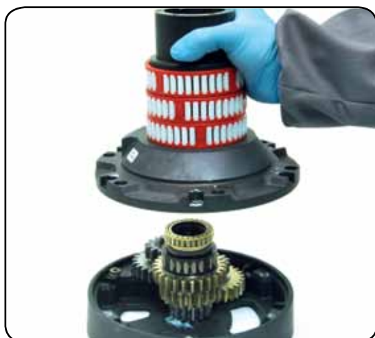
10. Remove the drum housing n°16. Attention! The gear assembly n°36 remains inside the drum housing
