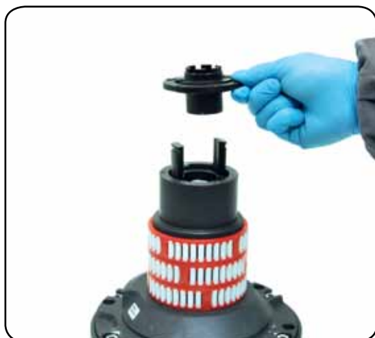
6. Remove the stripper arm housing n°21
