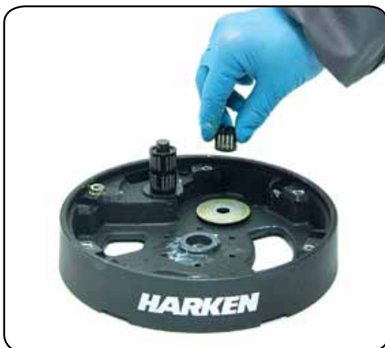
17. Remove the roller bearing n°12
