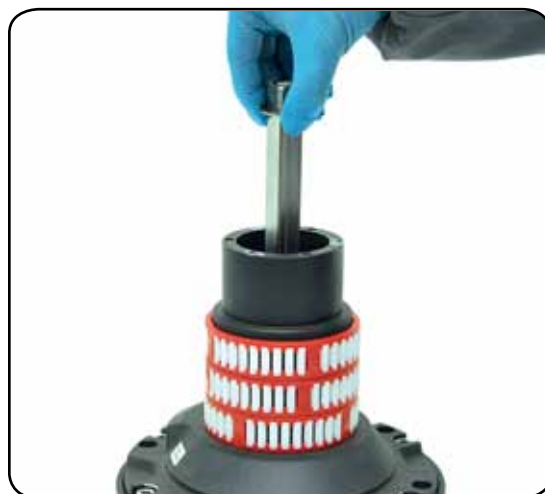
8. Slide out the central shaft n°19
