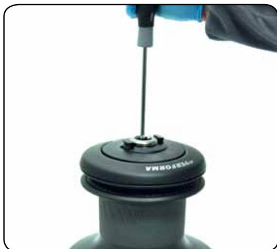
1. Unscrew the central screw ( \approx 2\text{Nm}/18\text{ in-lb} )
