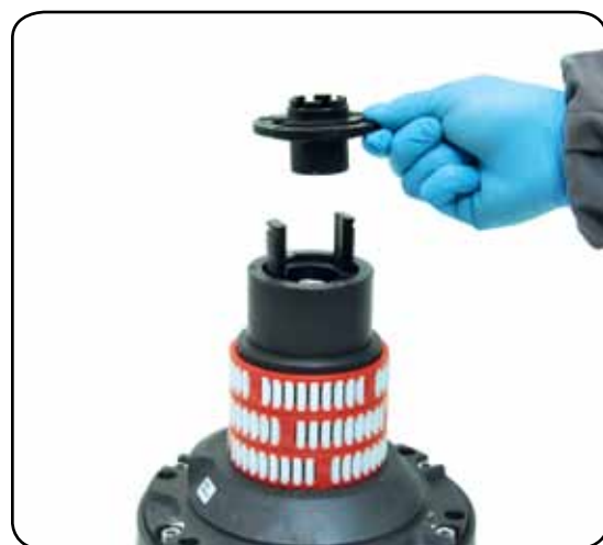
6. Remove the stripper arm housing n°21
