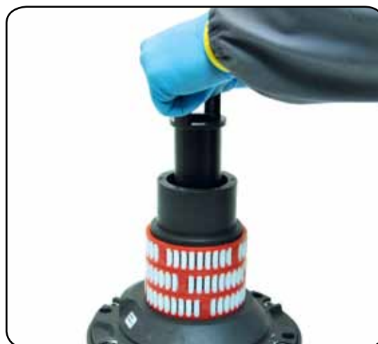
7. Slide out the assy clutch n°35
