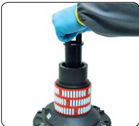
7. Slide out the assy clutch n°35
