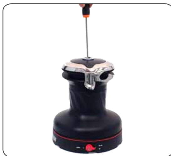
2. Unscrew the central screw ( \approx 2\text{Nm}/18\text{ in-lb} )
