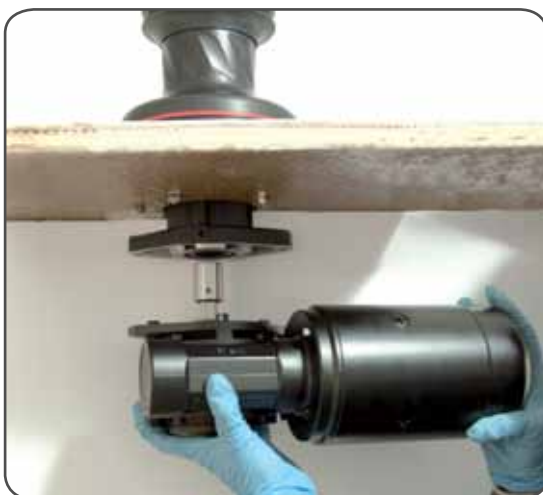
3. Position the reduction gear and motor
