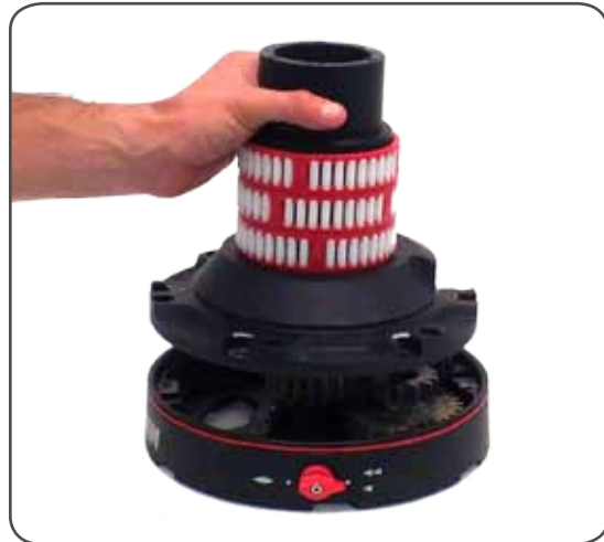
9. Remove the assy drum support n°13
