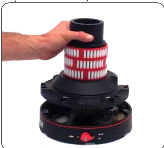
9. Remove the assy drum support n°13
