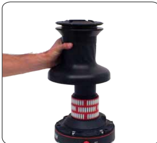
6. Lift off the drum n°20
