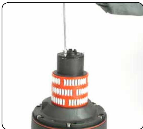
6. Completely unscrew the three screws n° 28
