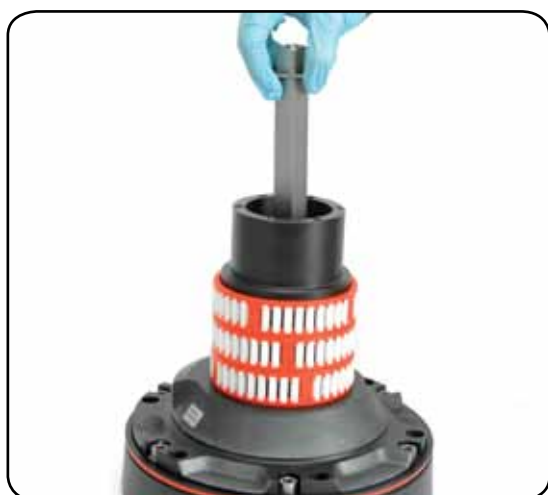
8. Slide out the central shaft n°19
