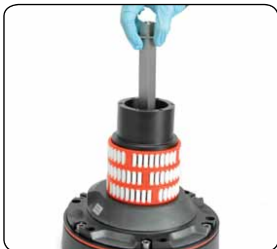
8. Slide out the central shaft n°19
