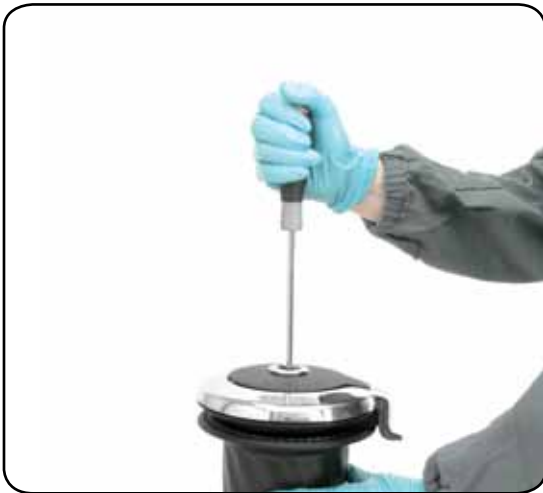
1. Unscrew the central screw (🔧2Nm/18 in-lb)
