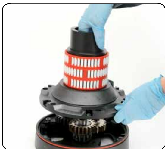
10. Remove the drum support n°16
