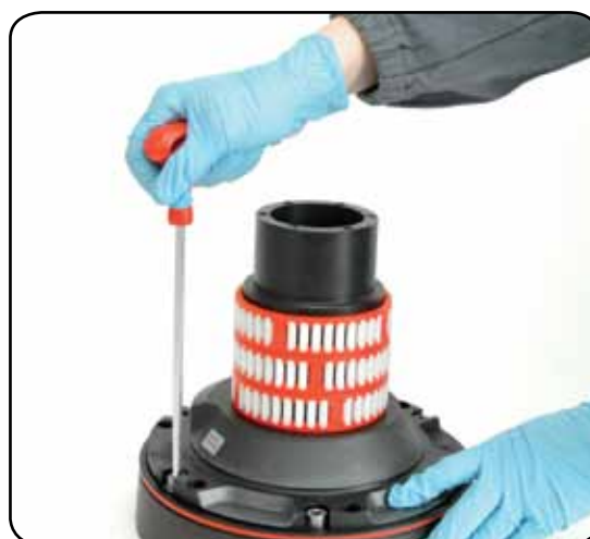
9. Unscrew the 6 hex screws n°17 ( \approx 20Nm/177 in-lb)
