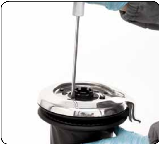
3. Unscrew the three screws n°28 (🔧4Nm/35 in-lb)
