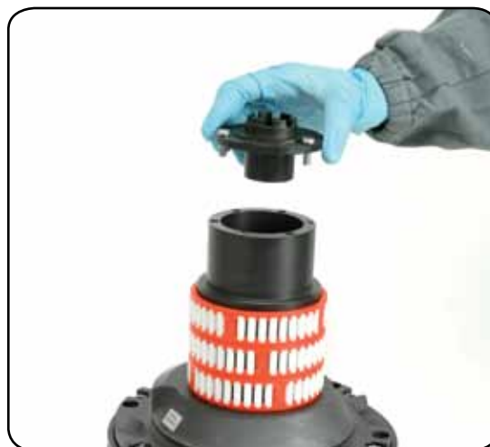
7. Remove the stripper arm housing n°21
