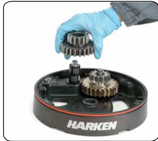
13. Remove the idler and pinion n°14
