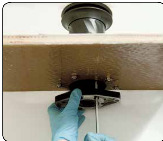
2. Tighten six M6 precote coated screws ( \approx 8 Nm/ 71 in-lb)
