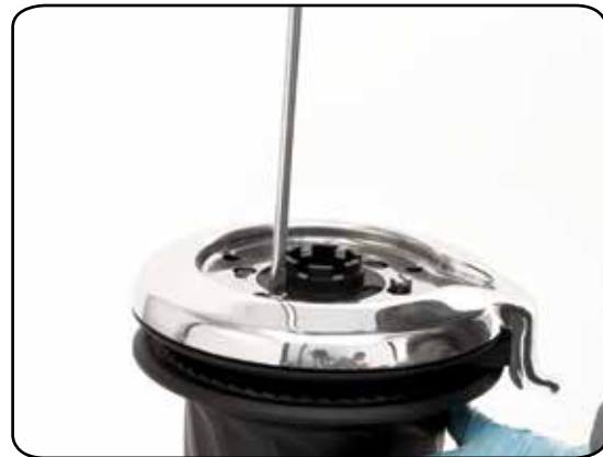
4. Unscrew the three screws ( \approx 4\text{Nm}/35\text{ in-lb} )
