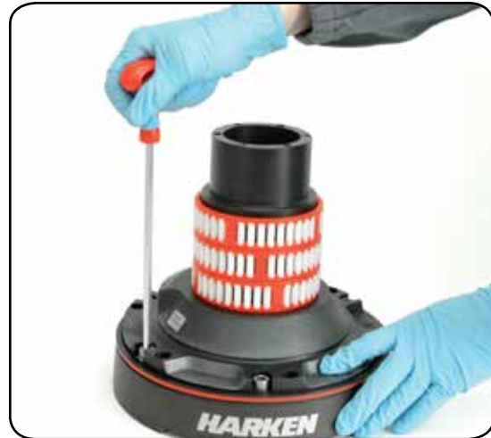
10. Unscrew the 6 hex screws ( 20Nm/177 in-lb)
