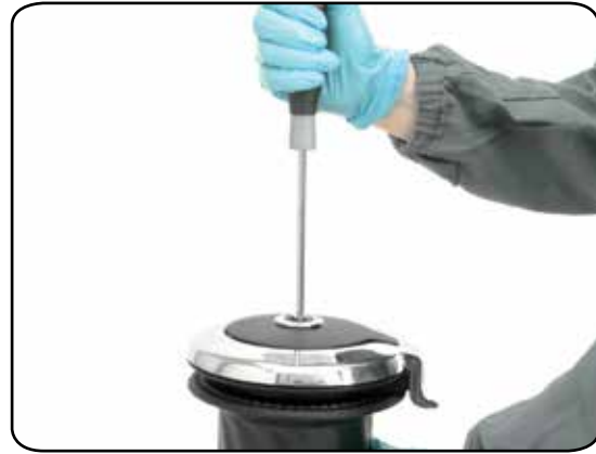
2. Unscrew the central screw ( \approx 2\text{Nm}/18\text{ in-lb} )
