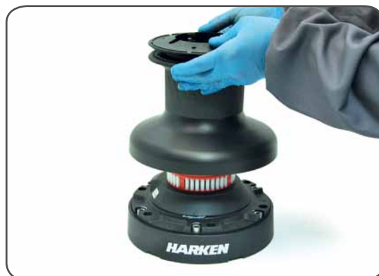
6. Lift off the drum n°23
