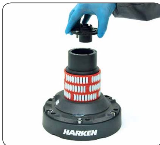
8. Remove the stripper arm support n°21
