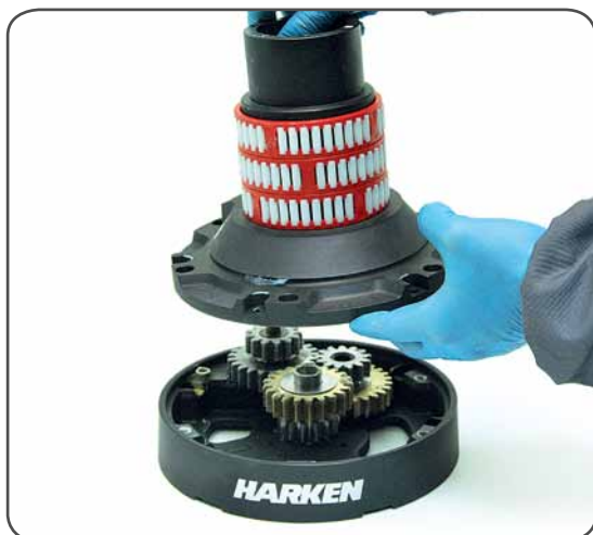
11. Remove the assy housing n°16
