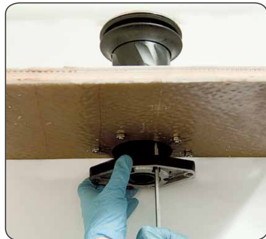
2. Tighten the six screws ( \approx 8 \text{ Nm} / 71 \text{ in-lb} )
