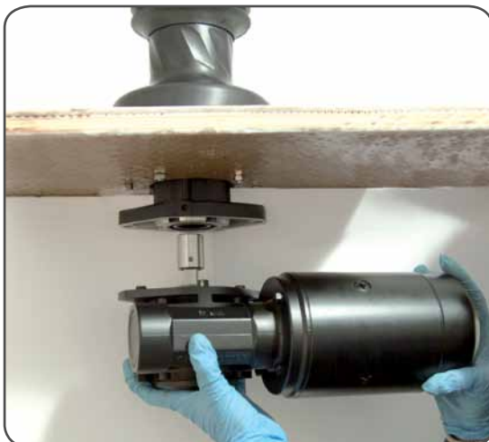
3. Position the reduction gear and motor
