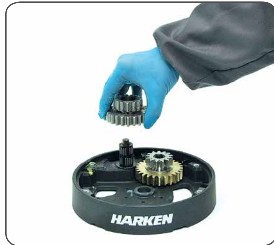
14. Remove the idler and pinion n°14.
