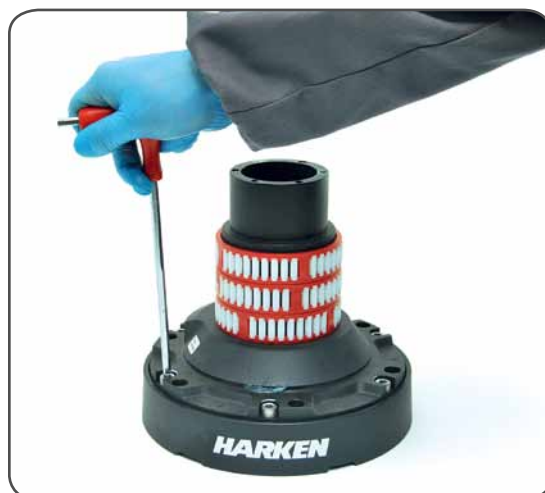
8. Remove the stripper arm support n°21
