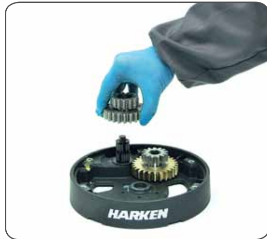
13. Remove the idler and pinion n°14.
