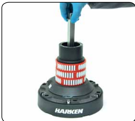
8. Slide out the central shaft n°19
