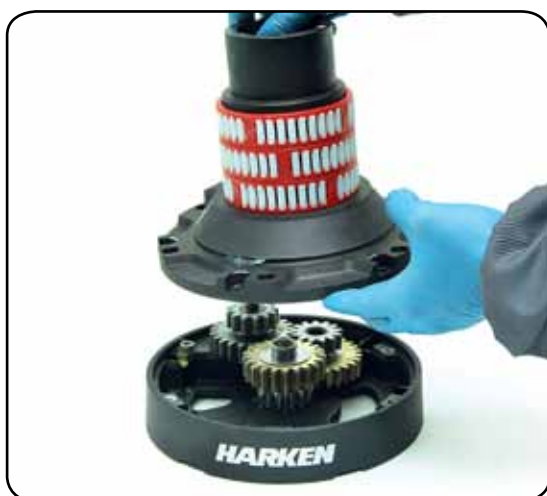
10. Remove the assy housing n°16
