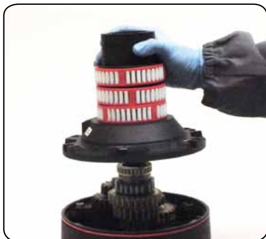
10. Remove the drum support n°16
