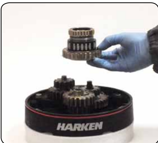
11. Remove the gear n°34, pawls carrier n°33, the bearings n°35 and 37 and the pin n°36 Important: washer n°7 may remain inside the drum support!
