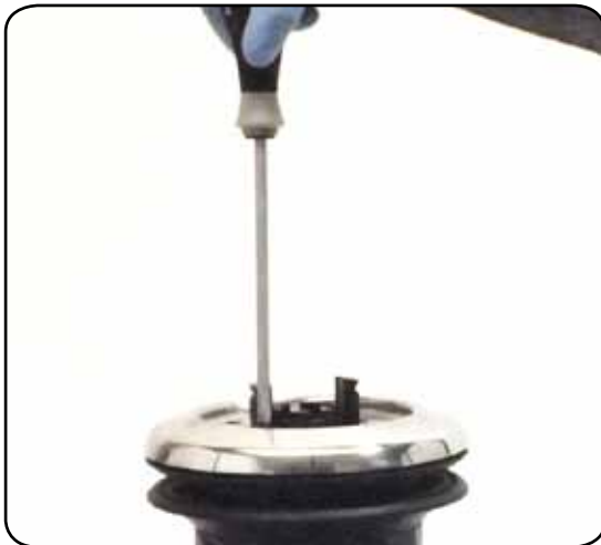
3. Unscrew the three screws n°28 (🔧4Nm/35 in-lb)
