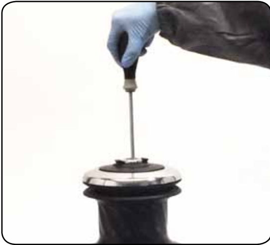
1. Unscrew the central screw (🔧2Nm/18 in-lb)
