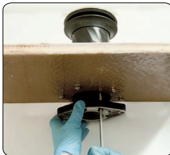
2. Tighten the six screws (⚙️ 8 Nm/ 71 in-lb)
