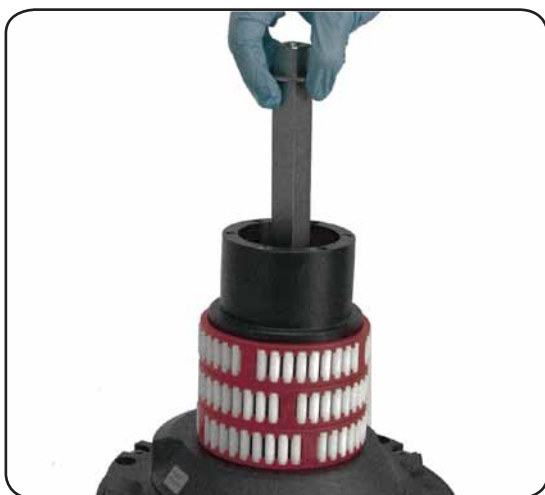
9. Slide out the central shaft n°19
