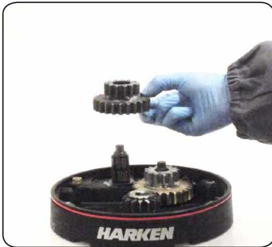
14. Remove the idler and pinion n°14
