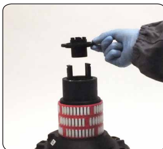
7. Remove the stripper arm housing n°21
