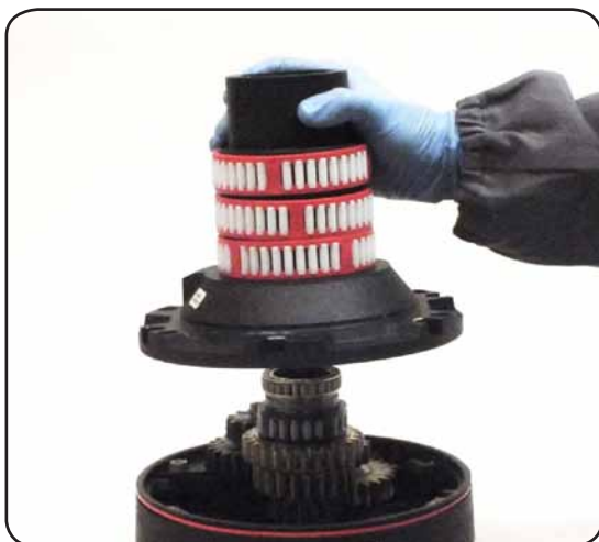
11. Remove the drum support n°16
