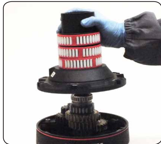
11. Slide out the drum support n°16
