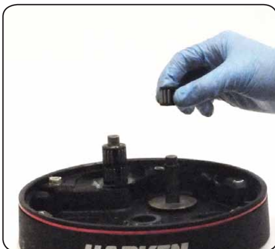
18. Remove the roller bearing n°12
