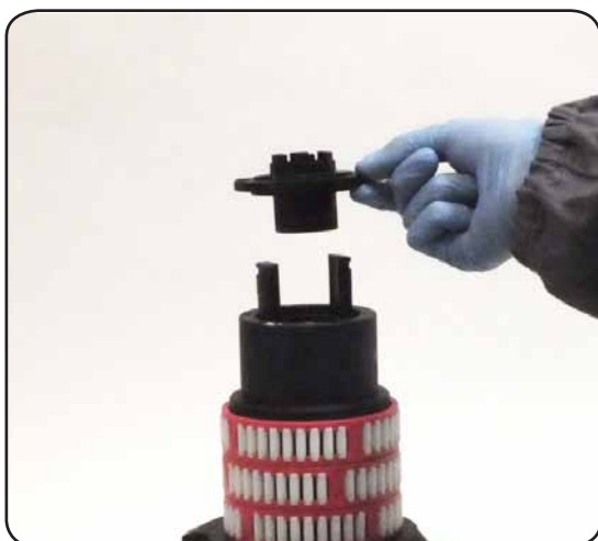
7. Remove the stripper arm housing n°21
