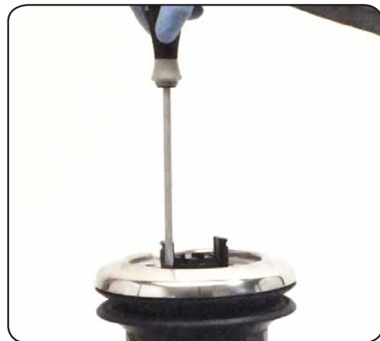
4. Unscrew the three screws n°28 ( \approx 4\text{Nm}/35\text{ in-lb} )
