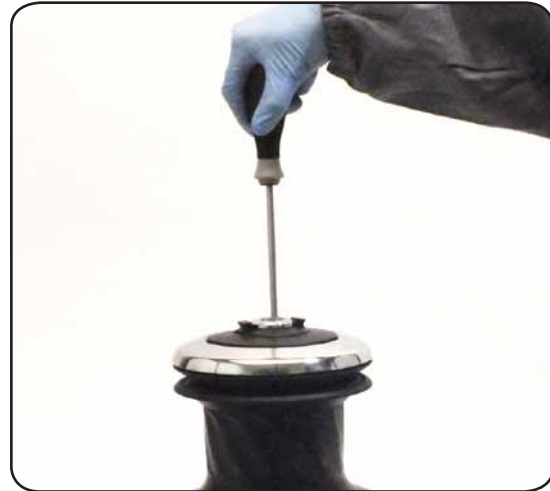
2. Unscrew the central screw ( \approx 2\text{Nm}/18\text{ in-lb} )
