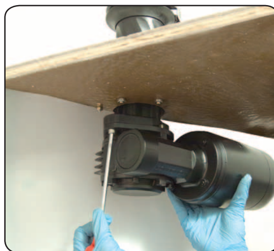
4. Tighten the two screws (⚙️ 8 Nm/ 71 in-lb). Be sure to align the flange.
