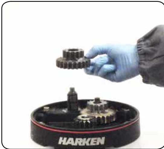
14. Remove the idler and pinion
