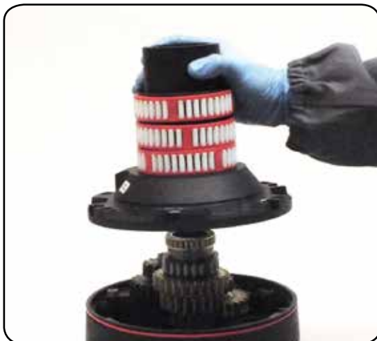
11. Remove the drum support
