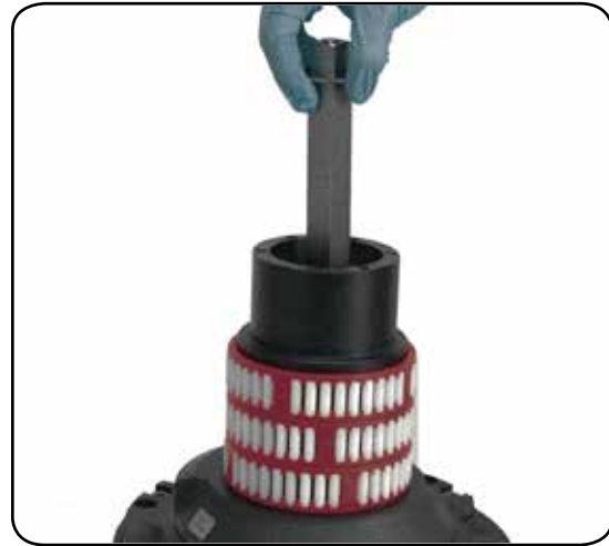
9. Slide out the central shaft
