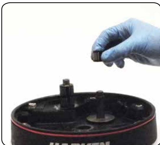
18. Remove the roller bearing
