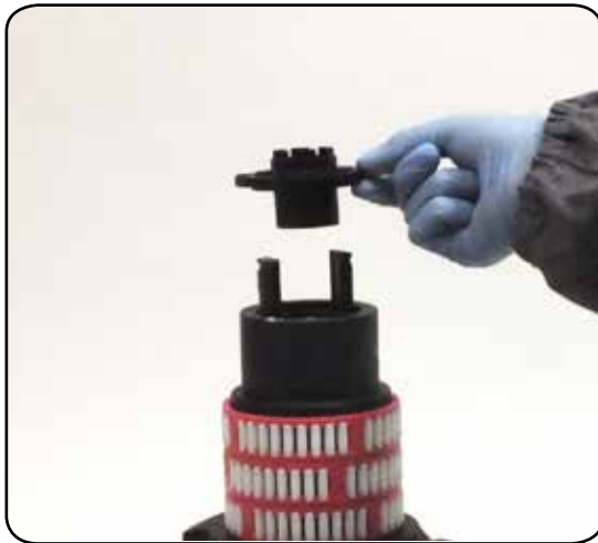
7. Remove the stripper arm housing
