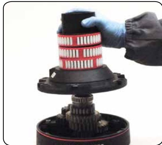
11. Slide out the drum support
