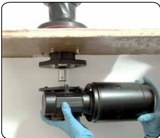
3. Position the reduction gear and motor
