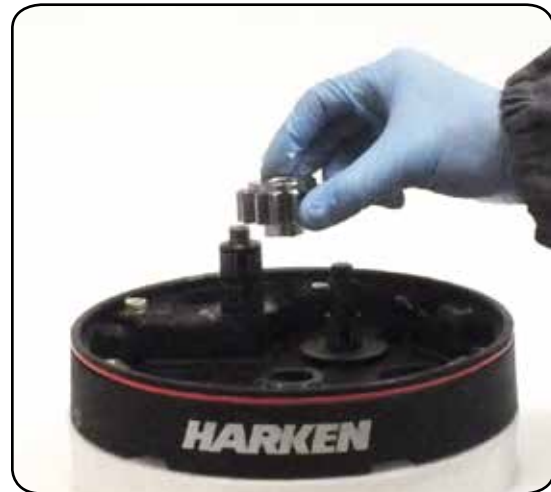
17. Remove the gear
