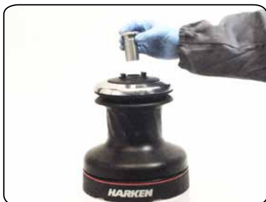
3. Slide off the assy socket and the cover
