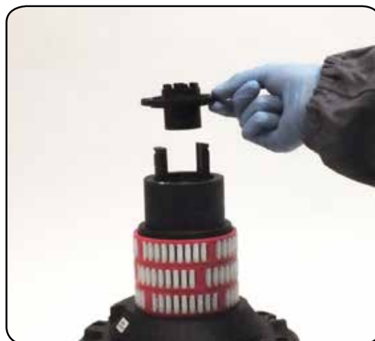
7. Remove the stripper arm housing
