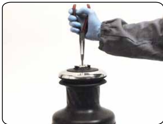
1. Pull out the disconnect rod
