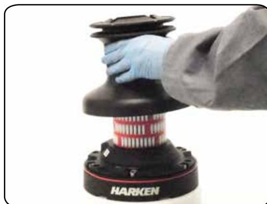
6. Lift off the drum
