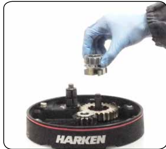
15. Remove the pawl carrier
