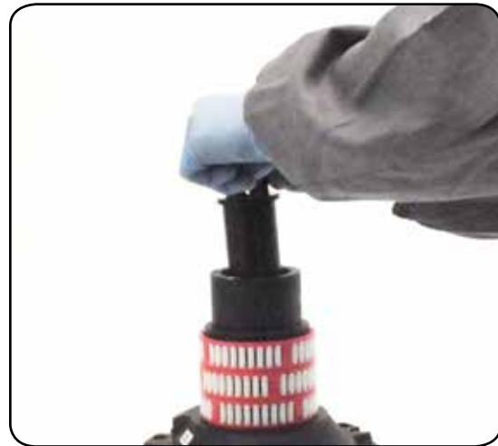
8. Slide out the assy clutch
