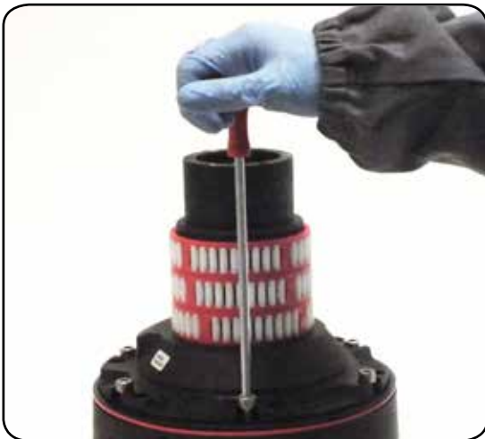
10. Unscrew the six hex screws ( \approx 20\text{Nm}/177\text{ in-lb} )
