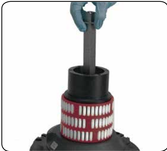
9. Slide out the central shaft
