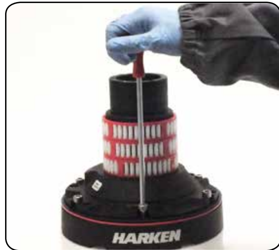
10. Unscrew the 6 hex screws ( \approx 20\text{Nm}/177\text{ in-lb} )
