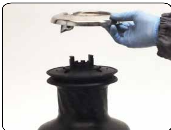
5. Remove the self-tailing arm by rotating and lifting it.
