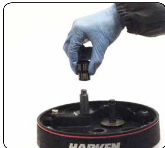
18. Remove roller bearings
