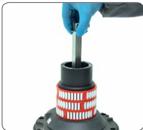
9. Slide out the central shaft n°19
