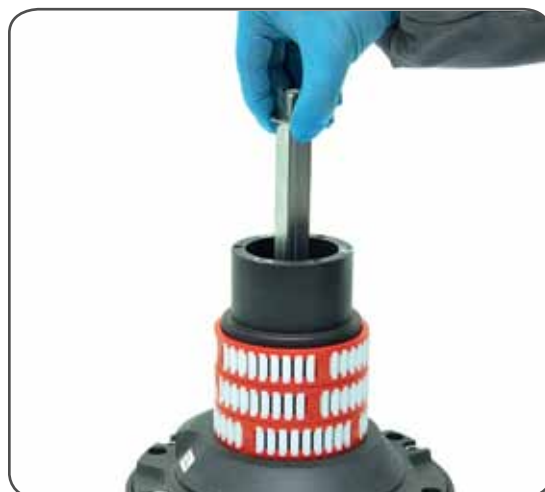
9. Slide out the central shaft n°19
