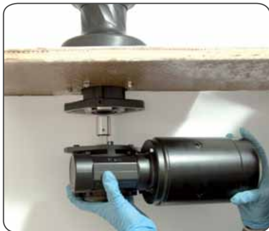
3. Position the reduction gear and motor
