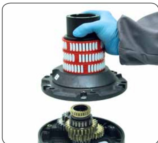
11. Remove the drum support n°16
