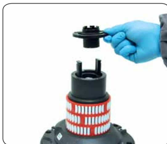
7. Remove the stripper arm housing n°21
