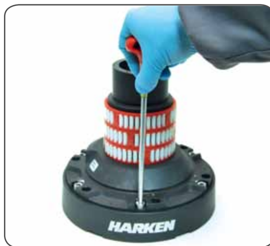
10. Unscrew the 6 hex screws n°17 ( \approx 20Nm/177 in-lb)
