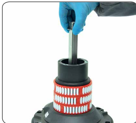
9. Slide out the central shaft n°19
