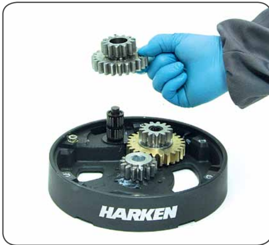
14. Remove the idler and pinion n°14
