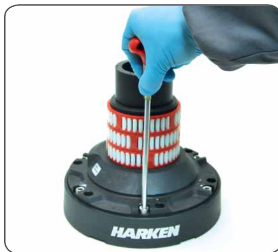
10. Unscrew the 6 hex screws n°17 (20Nm/177 in-lb)
