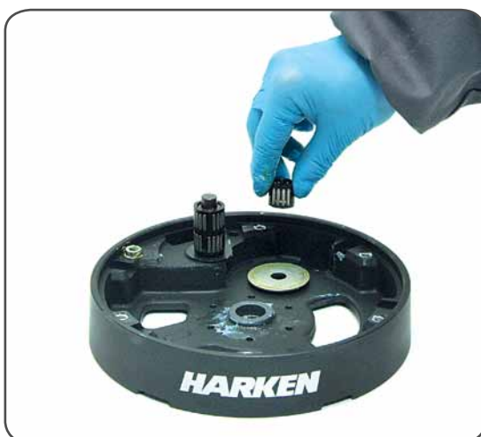
18. Remove the roller bearing n°12
