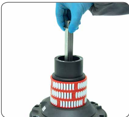
9. Slide out the central shaft n°19
