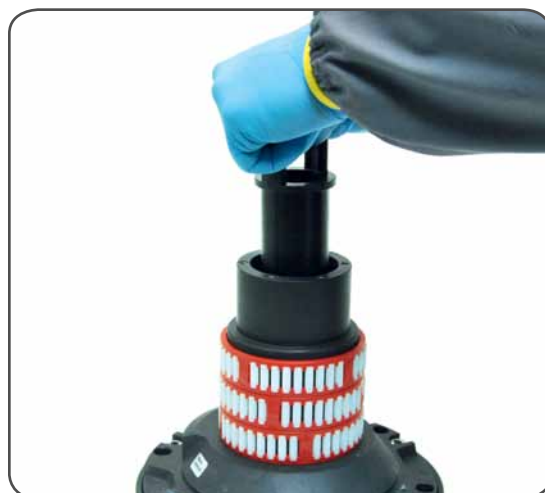
8. Slide out the assy clutch n°37
