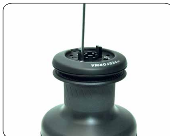
4. Unscrew the three screws n°27 ( \approx 4\text{Nm}/35\text{ in-lb} )
