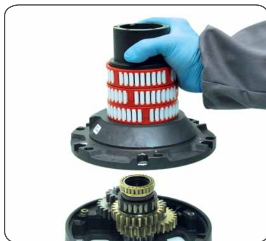
11. Slide out the drum support n°16
