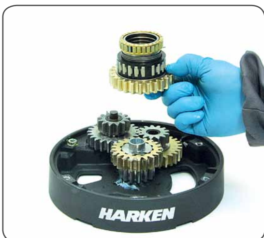
12. Remove the gear n°33, pawls carrier n°32, the bearings n°34 and 36 and the pin n°35 Important: washer n°7 may remain inside the drum support!
