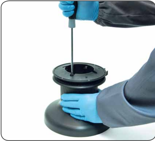
I. Unscrew the 4 screws n°25 ( \approx 4Nm/35 in-lb)
