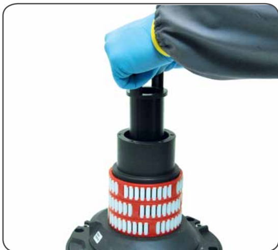
8. Slide out the assy clutch n°37
