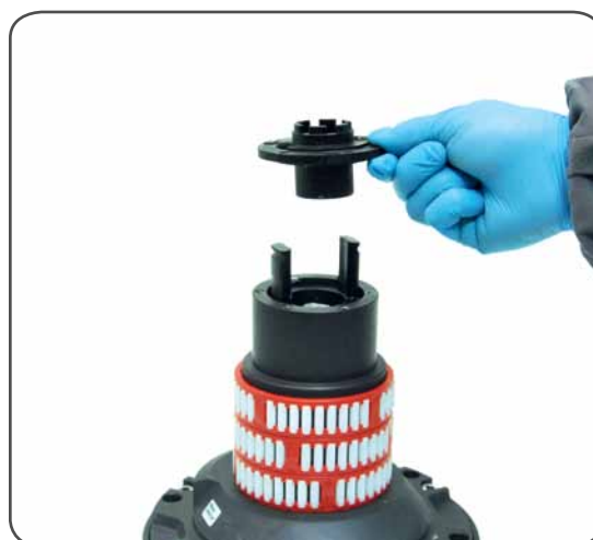
7. Remove the stripper arm housing n°21
