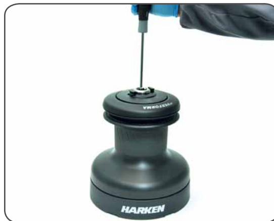
2. Unscrew the central screw ( \approx 2\text{Nm}/18\text{ in-lb} )
