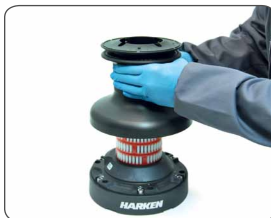
6. Lift off the drum n°23
