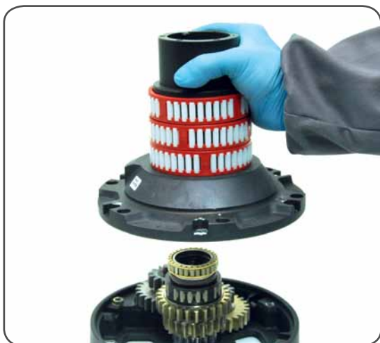
11. Remove the drum support n°16
