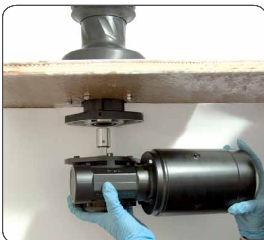
3. Position the reduction gear and motor
