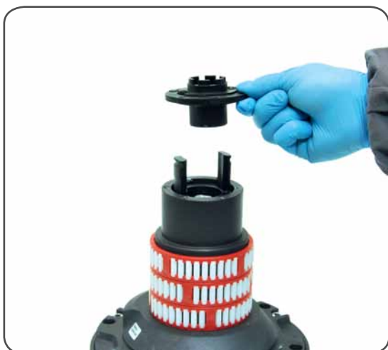
7. Remove the stripper arm housing n°21
