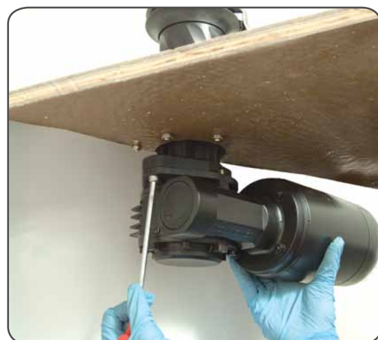
4. Tighten the two screws ( \approx 8 Nm/ 71 in-lb). Be sure to align the flange.
