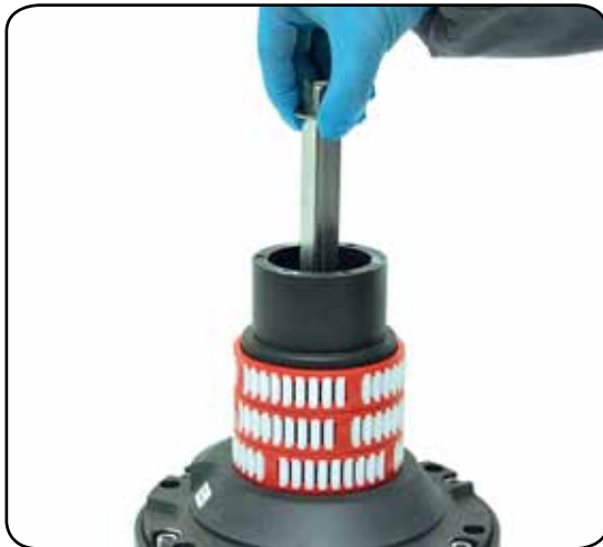
8. Slide out the central shaft n°19
