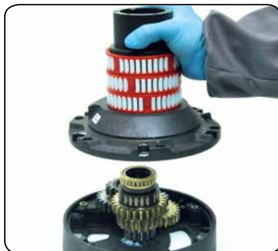
10. Slide out the drum housing n°16. Attention! The gear assembly n°29 remains inside the drum housing
