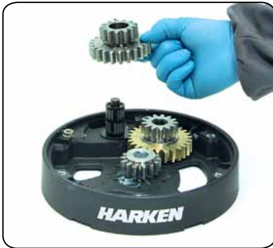
13. Remove the idler and pinion n°14
