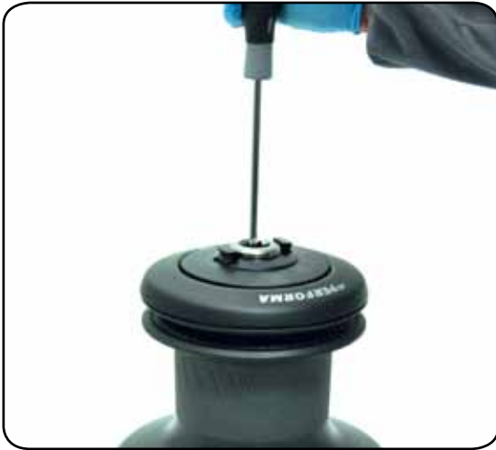
1. Unscrew the central screw ( \approx 2\text{Nm}/18\text{ in-lb} )
