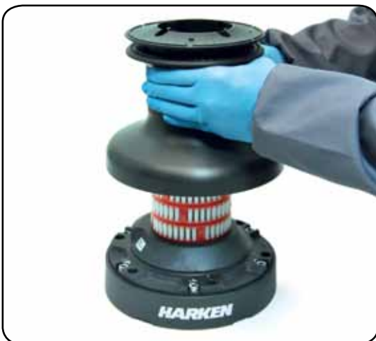
5. Lift off the drum n°23
