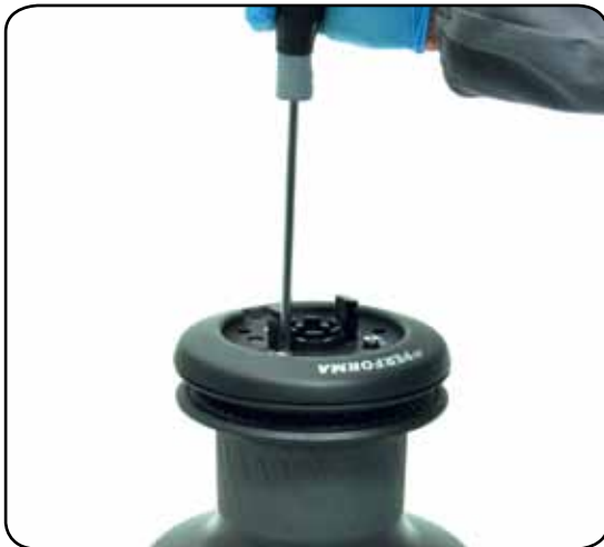
3. Unscrew the three screws n°26 ( \approx 4\text{Nm}/35\text{ in-lb} )
