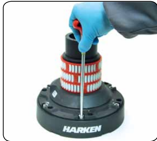
9. Unscrew the 6 hex screws n°17 (20Nm/177 in-lb)
