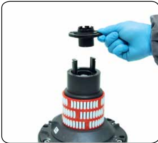
6. Remove the stripper arm support n°21
