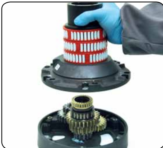
10. Remove the drum housing n°16
