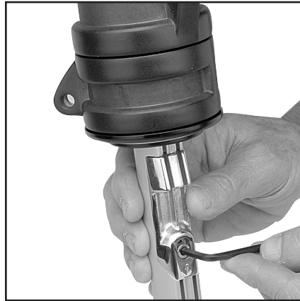
Loosen screw one revolution only.
