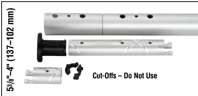
53/8"-4" (137-102 mm) Do not use plastic bushing above top connector. Cut connector right at cross formed by glue dispersion channels. Use single foil screw in top foil only.
