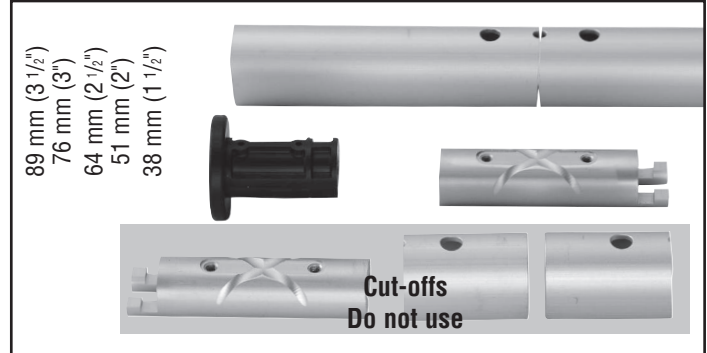
89 – 38 mm (3 1/2" – 1 1/2") Shorten top foil and adjoining full length foil so two (2) screws are used to assemble joint instead of four (4). Do not use plastic bushings above top connector.
