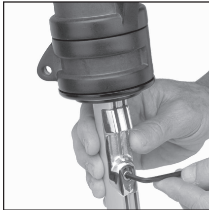
Loosen screw one revolution only .
