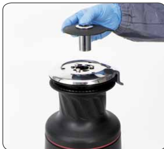
2. Slide off the assy socket n°26 and the cover n°9
