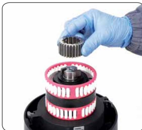
8. Lift off the gear n°17
