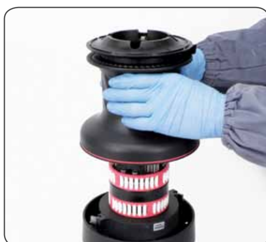
4. Lift off the drum n°22
