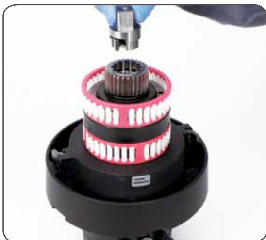
7. Slide out the pawls carrier n°16
