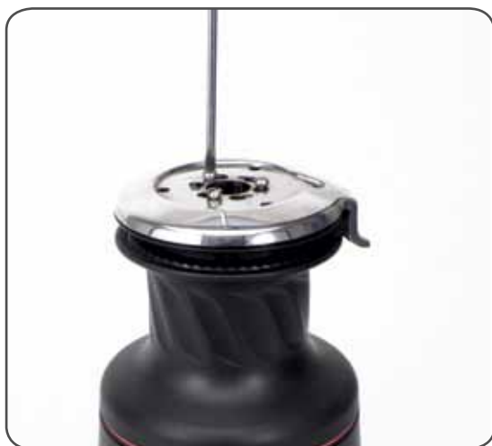
3. Unscrew the three screws n°20 (4Nm/35 in-lb) and remove the self-tailing arm n°7 by rotating and lifting it.
