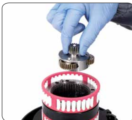
10. Slide out the first planetary assy n°19, the ring gear n°4, the o-ring n°8 and the pinion n°2.
