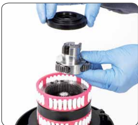
9. Remove the second planetary assy n°17 and remove flange. Pay attention to the o-ring in the ring gear.
