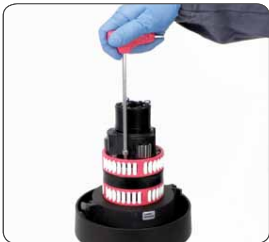
5. Unscrew the 6 hex screws n°14 (20Nm/177 in-lb)
